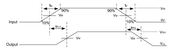
Notes: 1.  $V_{OL}$  and  $V_{OH}$  are typical output drop that occur with the output load.
