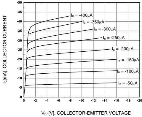
Figure 1. Static Characteristic
