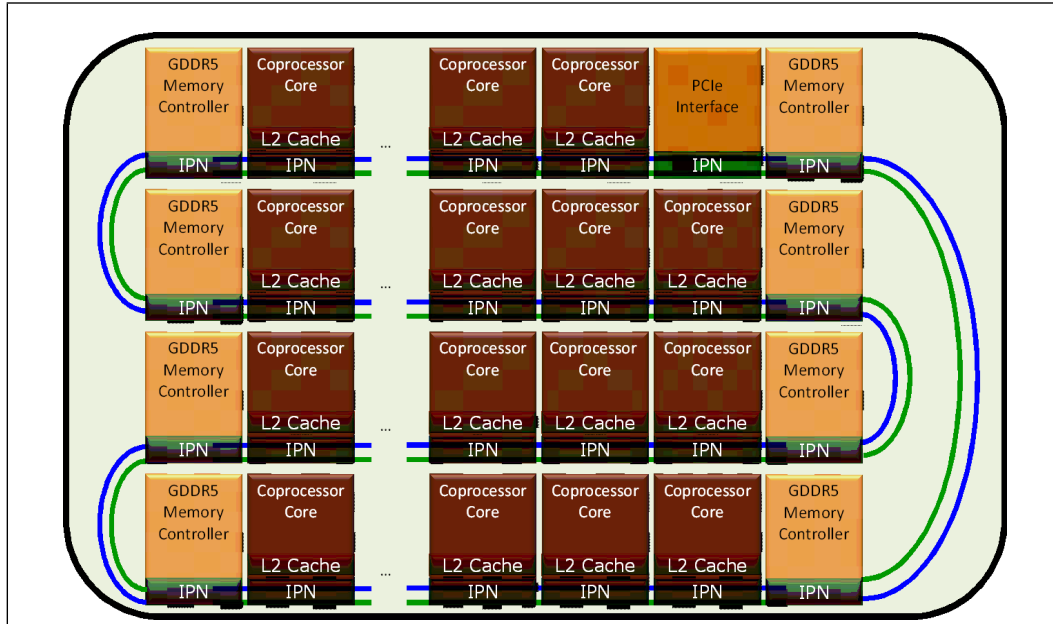
Figure 2-4. Intel® Xeon Phi™ Coprocessor Silicon Layout
