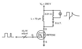
Fig. 11 - Reverse Recovery Parameter Test Circuit
