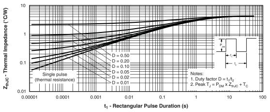
Fig. 5 - Maximum Thermal Impedance Z<sub>thJC</sub> Characteristics (FULL-PAK)
