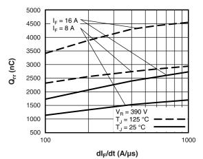
Fig. 10 - Typical Stored Charge vs. dl<sub>F</sub>/dt
