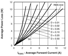
Fig. 8 - Forward Power Loss Characteristics
