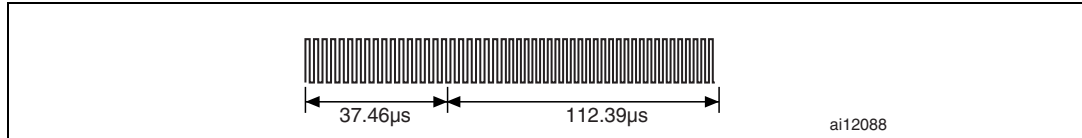
Figure 45. End of frame, high data rate, two subcarriers
