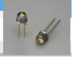
L9437 is an infrared LED developed for optical encoders. By improving the aspherical lens used with the previous type L8506, we have achieved an even more highly collimated beam of near infrared light. The lead pin of L9437 has no step piece that is usually formed at the lead base brazed to the package, thus eliminating the restriction in printed circuit board design.
