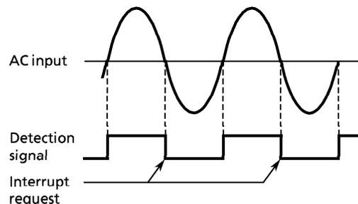
Figure 3-25. Detection Signal
