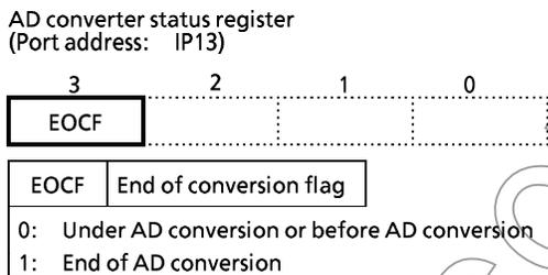
Figure 3-18. AD converter status register
