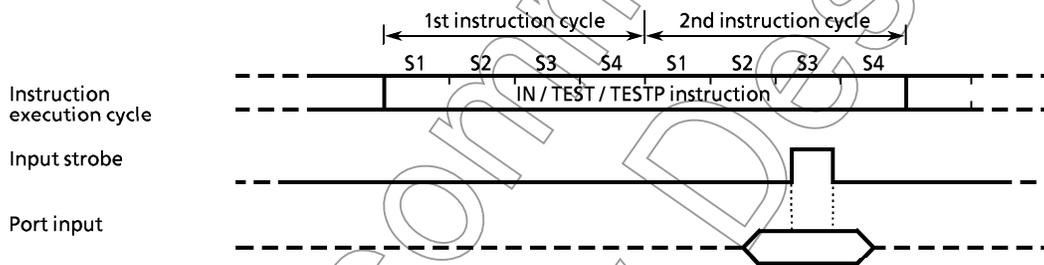
Figure 3-1. Input Timing
