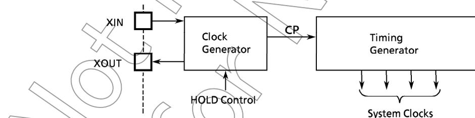
Figure 2-14. Clock Generator and Timing Generator
