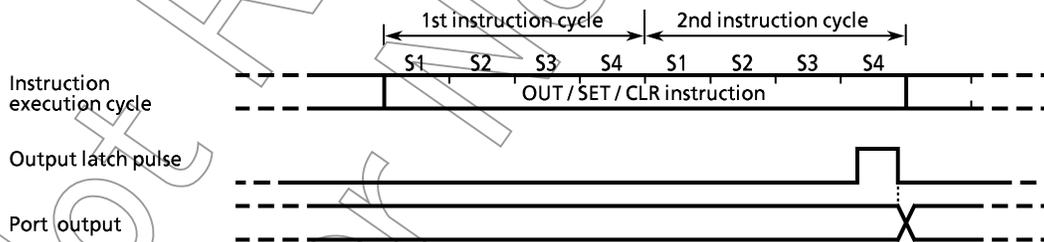
Figure 3-2. Output Timing
