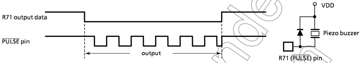
Figure 3-22. Circuit Example of Buzzer Pulse and Timing
