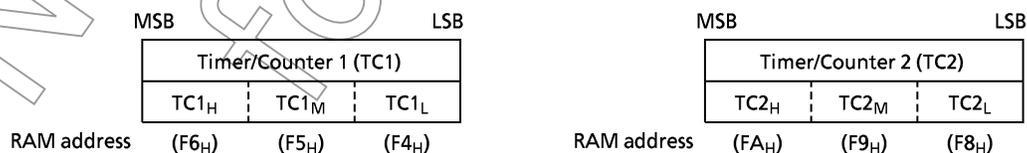
Figure 2-8. Count Registers of the Timer/Counters (TC1, TC2)
