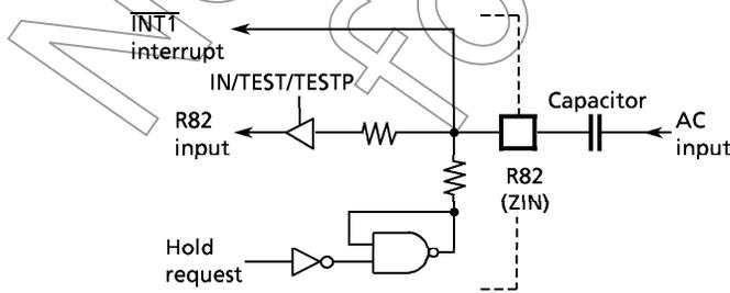
Figure 3-24. Zero-cross Detector
