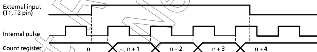
Figure 3-14. Pulse Width Measurement Mode Timing chart
