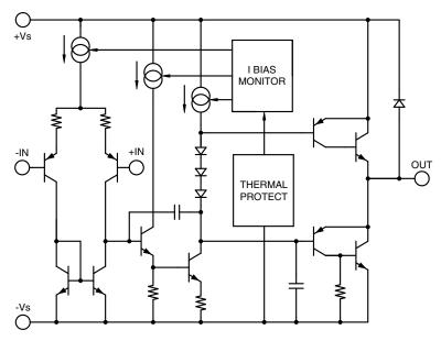
FIGURE 1. Equivalent schematic (one channel)
