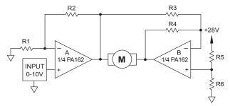
FIGURE 3. BI-DIRECTIONAL SPEED CONTROL FROM A SINGLE SUPPLY.
