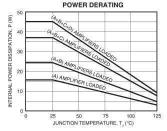
ratings are based on two separate dual monolithic power op amps on one integrated copper heat slug. Amps A and B are combined on one monolithic die while amps C and D are combined on the other. This multi chip configuration provides superior thermal performance by isolating each of the dual amplifiers. When loading either of the dual amplifiers it is possible to achieve better thermal performance by loading any combination of amplifiers (A or B) + (C or D).
