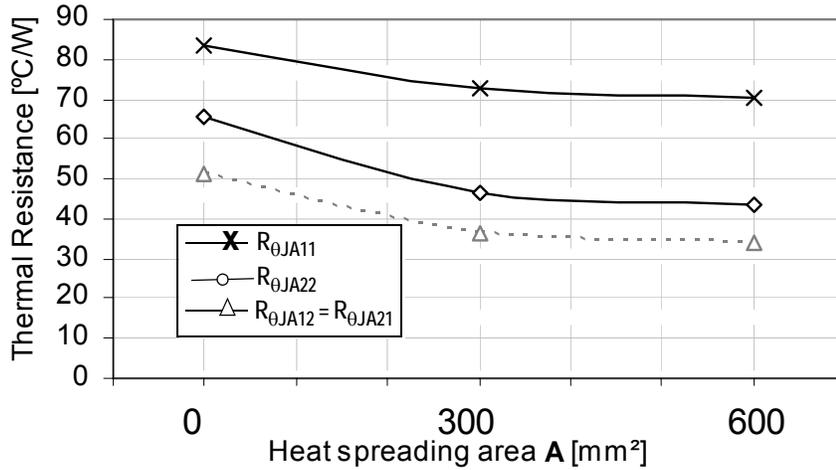
Figure 46. Device on Thermal Test Board R<sub>θJA</sub>
