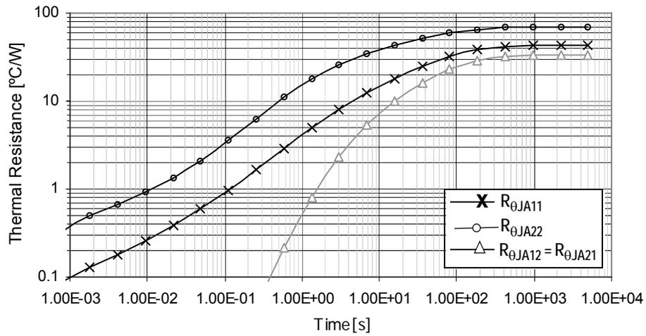
Figure 47. Transient Thermal Resistance R<sub>θJA</sub>,
