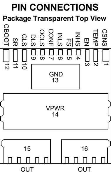
**Figure 3. Pin Connections**
