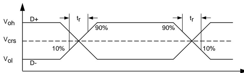
Figure 9 USB Data Signal Timing and Voltage Level
