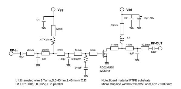
RoHS Compliance, Silicon MOSFET Power Transistor 175MHz,520MHz,2W
