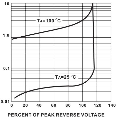
Fig.3 TYPICAL PEAK REVERSE CHARACTERISTICS
