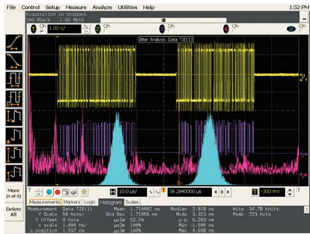
Figure 7. Performing jitter analysis on FlexRay signals is easy with Agilent EZJIT jitter analysis software
