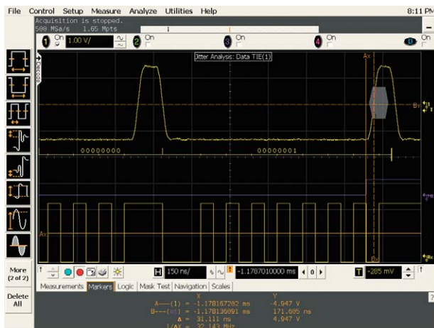
Figure 10. Timing measurements on the errant FlexRay pulse reveals that a BSS pulse occurred nearly one bit period early
