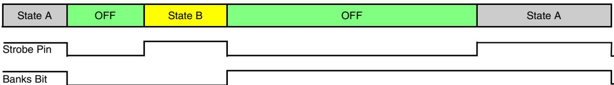
If strobe pin is 1, configuration is defined by BANKS. BANKS is toggled at each falling edge of the strobe pin.
