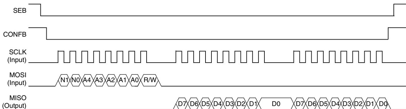
Figure 5. Read Operation in Configuration Mode (N[1:0] = 01)
