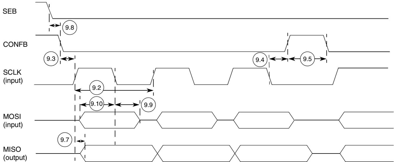
Figure 41. Digital Interface Timing Diagram in Configuration Mode
