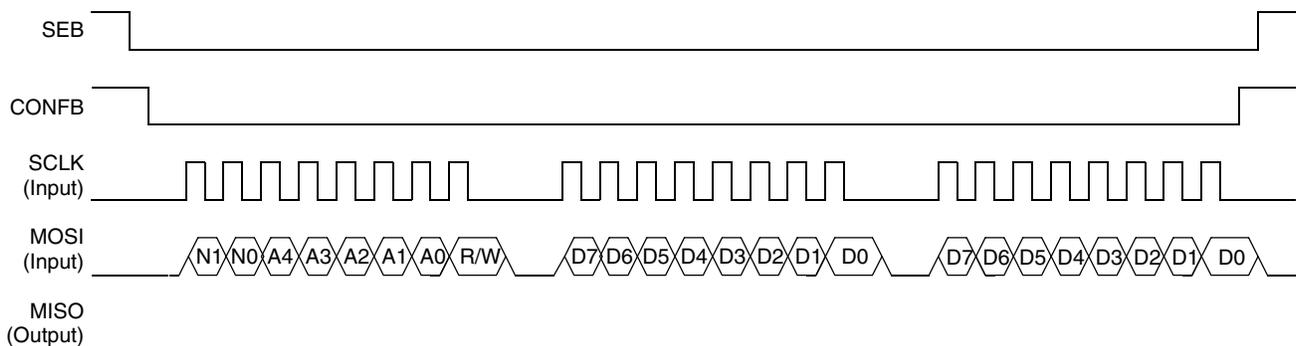
Figure 4. Write Operation in Configuration Mode (N[1:0] = 01)
