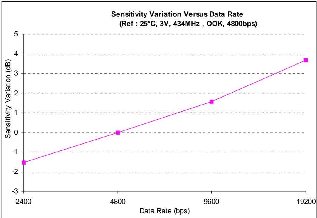
Figure 38. OOK Sensitivity Variation Versus Data Rate
