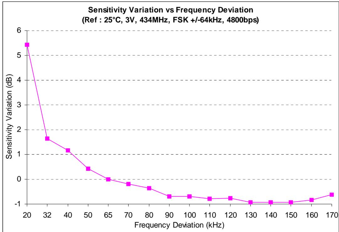
Figure 40. FSK Sensitivity Variation Versus Frequency Deviation
