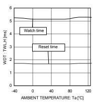
Fig.12 WDT Time vs. Temperature  $(CT=0.01\mu F)$
