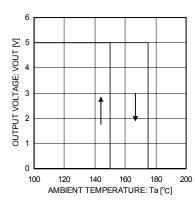
Fig.8 Thermal Shutdown Circuit Characteristics
