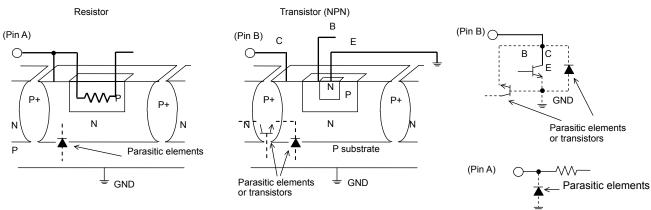
Example of Simple Monolithic IC Architecture
