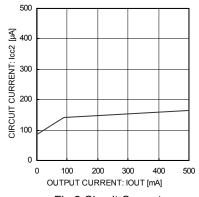
Fig.2 Circuit Current
