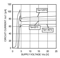
Fig.1 Circuit Current
