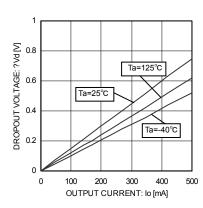
Fig.5 Dropout Voltage
