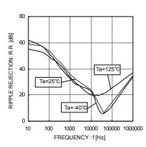
Fig. 6 Ripple Rejection
