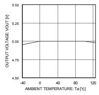
Fig. 7 Output Voltage Temperature Characteristics
