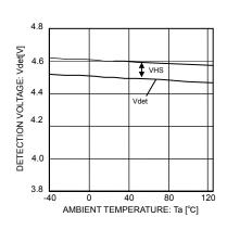
Fig.11 Reset Detection Voltage vs. Temperature
