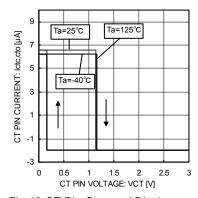
Fig.10 CT Pin Charge / Discharge Current (Vcc=5V)
