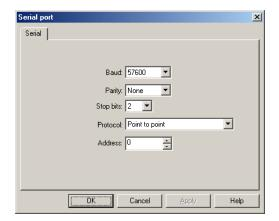
Make sure the serial cable is connected from the host computer's COM port to the DK Board. Set the serial interface parameters according to the default settings of 57600, None, 2, Point to point, 0. Click OK to attempt a connection and proceed to the Axis Setup Wizard. If no connection is made the Interface selection dialog will be displayed again allowing you to modify the interface parameters or run in demo mode.
