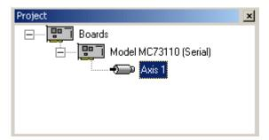
The Project window displays the available DK Board's and axes in a tree format. Double-clicking on a board or axis will display the properties dialog for that item.
