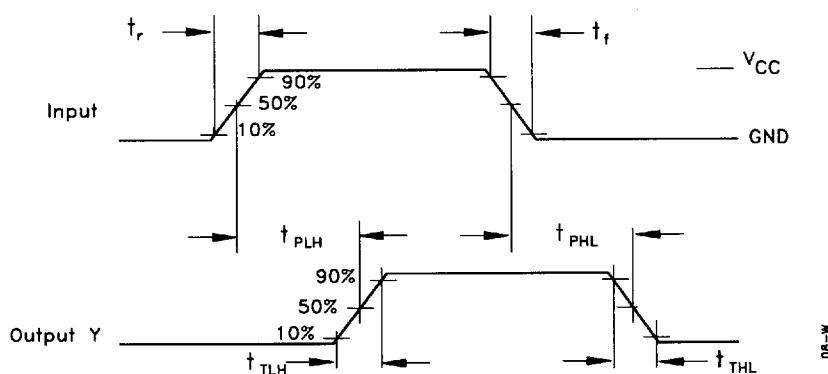
Input and Output Threshold Voltage: V<sub>T</sub> = 50% V<sub>CC</sub> for HC,
