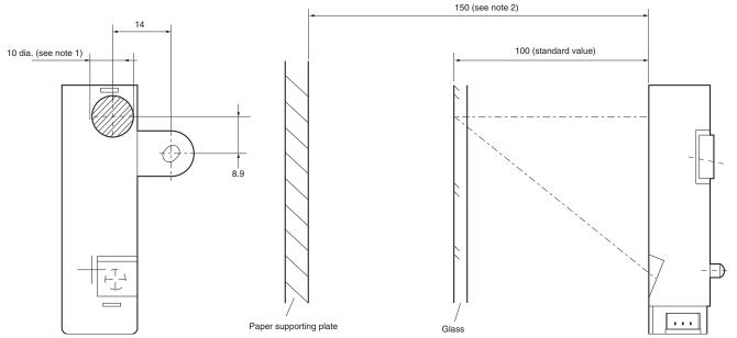
Note: 1. The part with oblique lines indicates the paper sensing area of the EY3A-110-A, which is practically determined by the diameter of the beam and its tolerance.
