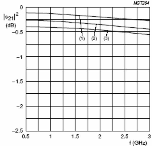
(1)  $I_F = 10 \text{ mA}$ .      (2)  $I_F = 1 \text{ mA}$ .      (3)  $I_F = 0.5 \text{ mA}$ .
