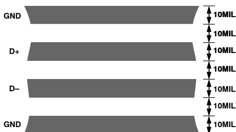
Figure 18. Arrangement of Signal Tracks
