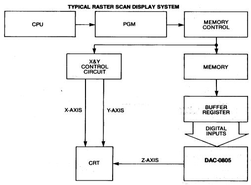
The DAC-0805 is particularly useful in raster scan display systems. The above system functions as an intelligent peripheral to the host CPU, and drives a standard television monitor.
