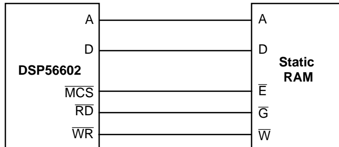
Figure 5-1 Static RAM Connection Diagram
