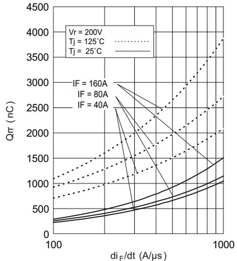
Fig. 8 - Typical Stored Charge vs.  $di_F/dt$
