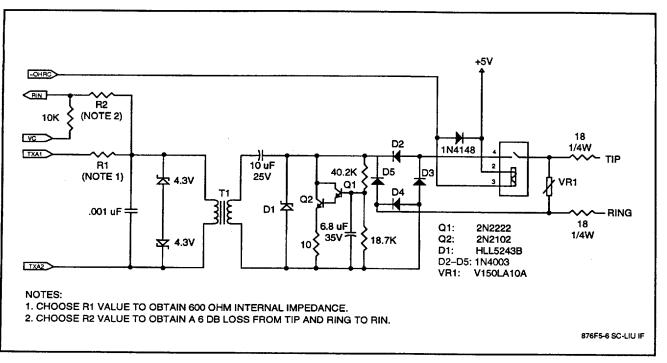
Figure 11. Typical Line Interface
