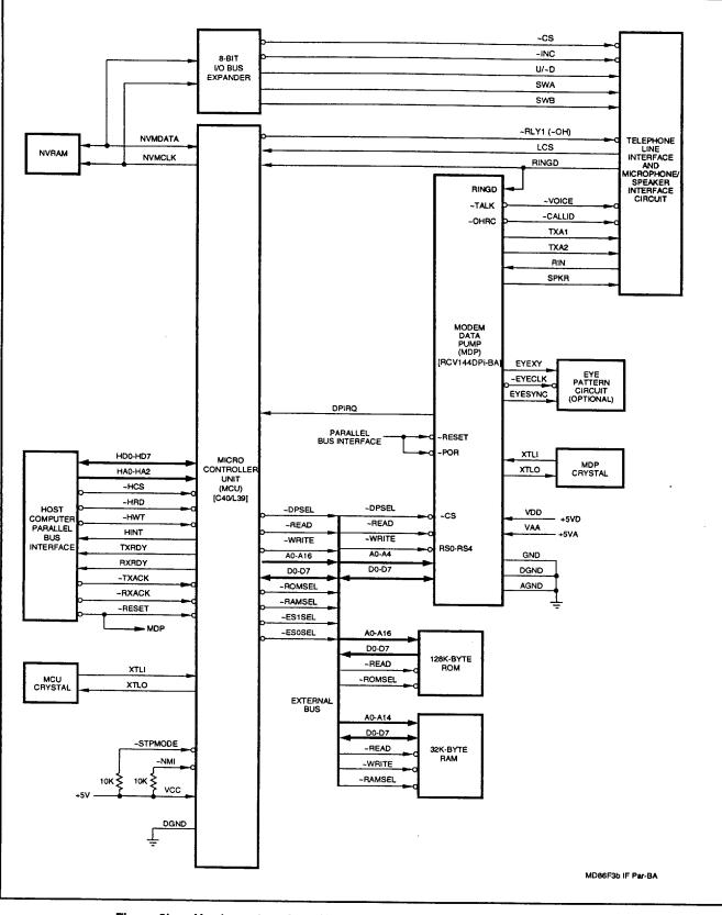
Figure 3b. Hardware Interface Signals - Parallel Interface with Business Audio
