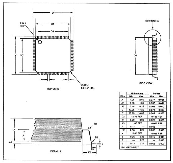
Figure 14d. Package Dimensions - 80-Pin PQFP
