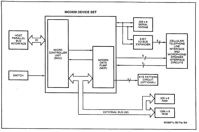
Figure 1c. Block Diagram - Parallel Interface with Business Audio
