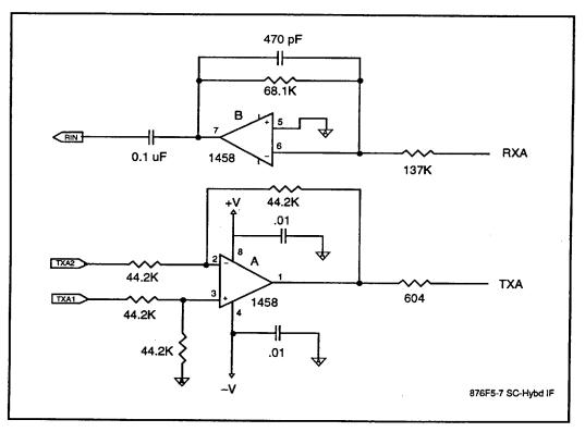
Figure 12. Typical Interface to External Hybrid
