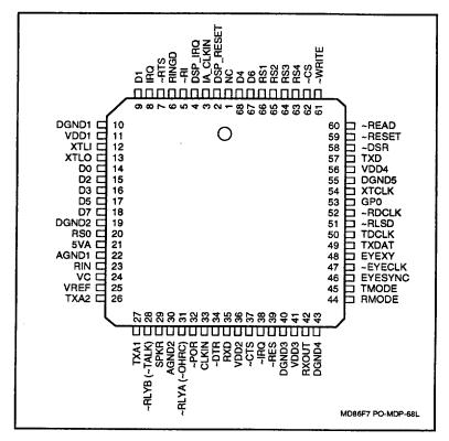
Figure 6. MDP Pin Signals - 68-Pin PLCC
