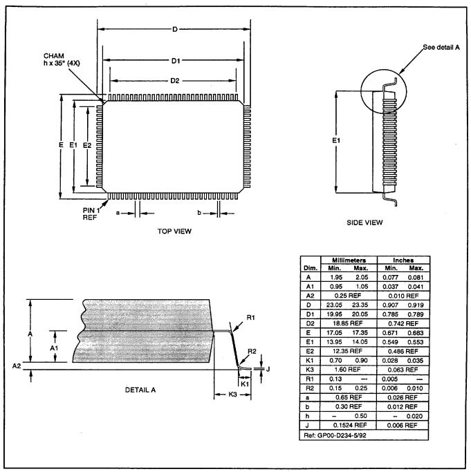
Figure 14c. Package Dimensions - 100-Pin PQFP
