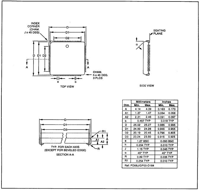
Figure 14a. Package Dimensions - 68-Pin PLCC
