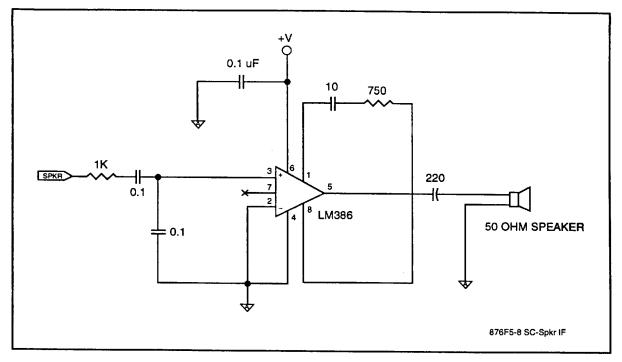
Figure 13. Typical External Speaker Circuit
