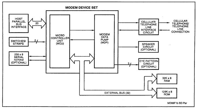
Figure 1b. Block Diagram - Parallel Interface
