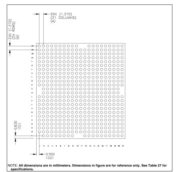
Figure 20. Surface-mount BGA2 Package - Bottom View
