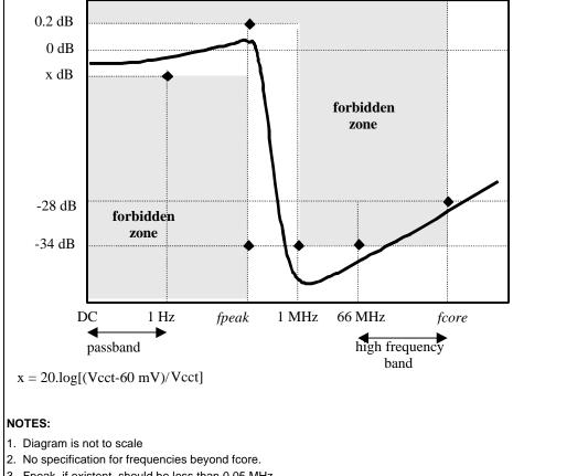
Figure 25. PLL Filter Specifications
