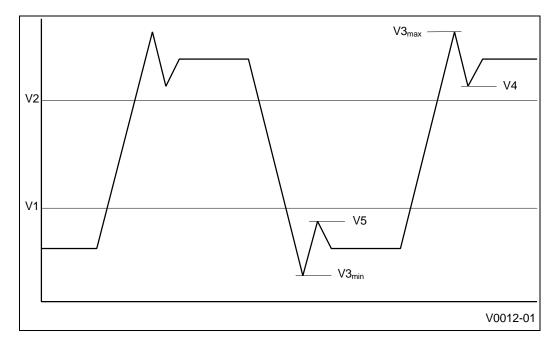
Figure 15. BCLK/PICCLK Generic Clock Waveform
