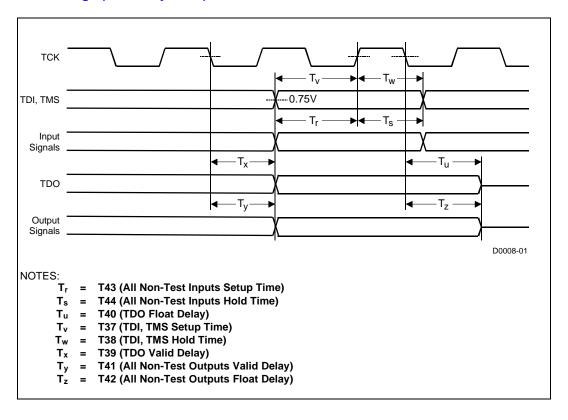
**Figure 12. Test Reset Timings**
