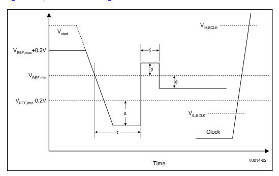
Figure 17. High to Low, GTL+ Receiver Ringback Tolerance
