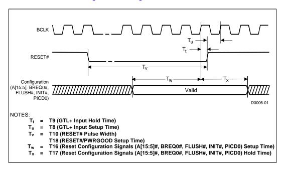
Figure 10. Power-on Reset Timings
