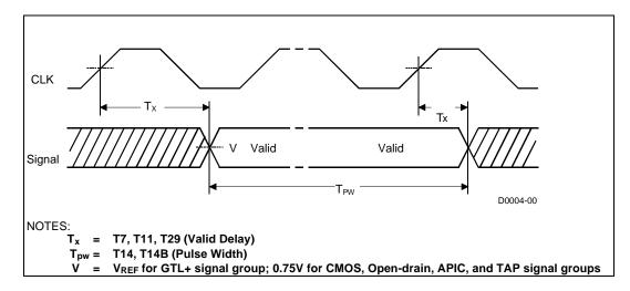
Figure 8. Setup and Hold Timings
