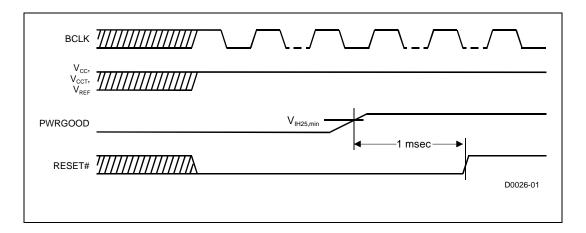
The PWRGOOD signal, which must be supplied to the processor, is used to protect internal circuits against voltage sequencing issues. The PWRGOOD signal should be driven high throughout boundary scan operation.
