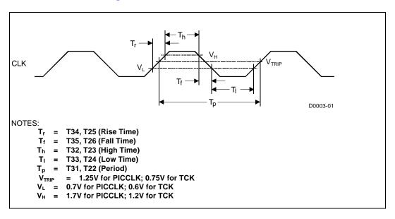
Figure 6. BCLK Timing Waveform
