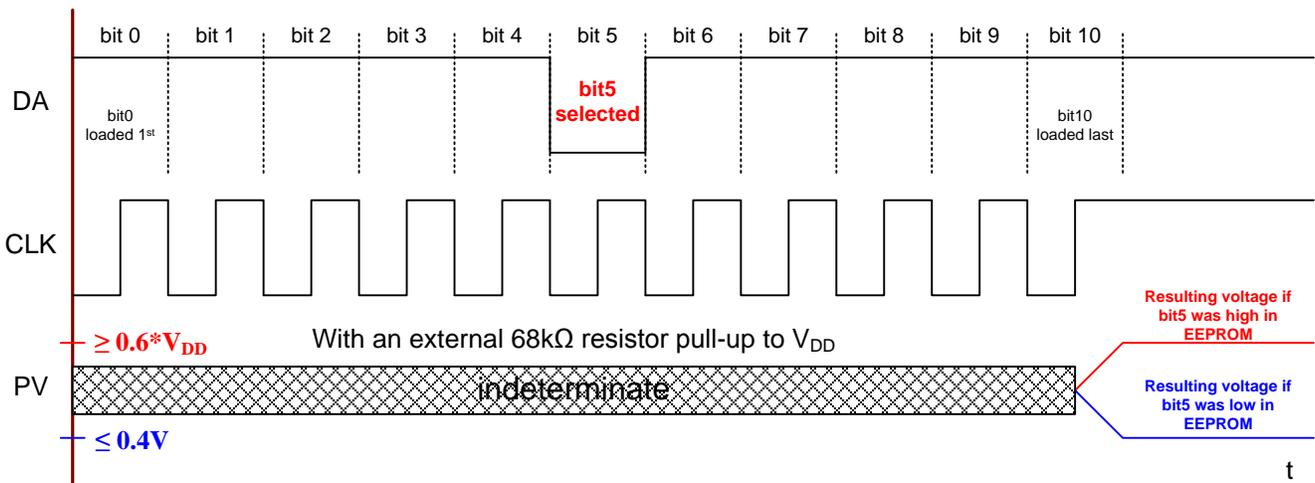
Figure 12 – Timing diagram to read bits from EEPROM
