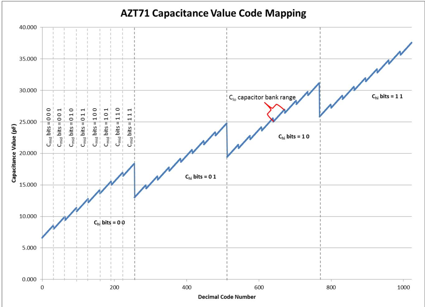
Figure 4 – AZT71 Capacitance Value Mapping
