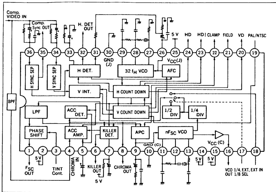
System Block Diagram to which  $\mu$ PC1860 is Applied
