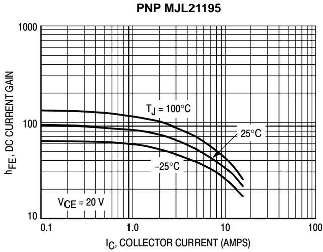
Figure 3. DC Current Gain,  $V_{CE} = 20\text{ V}$
