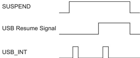
As the device has a remote wake up function it can wake-up the USB Host by sending a wake-up pulse through RMWK (bit 1 of the USC register). Once the USB Host receives a wake-up signal from the devices, it will send a Resume signal to the device. The timing is as follows:
