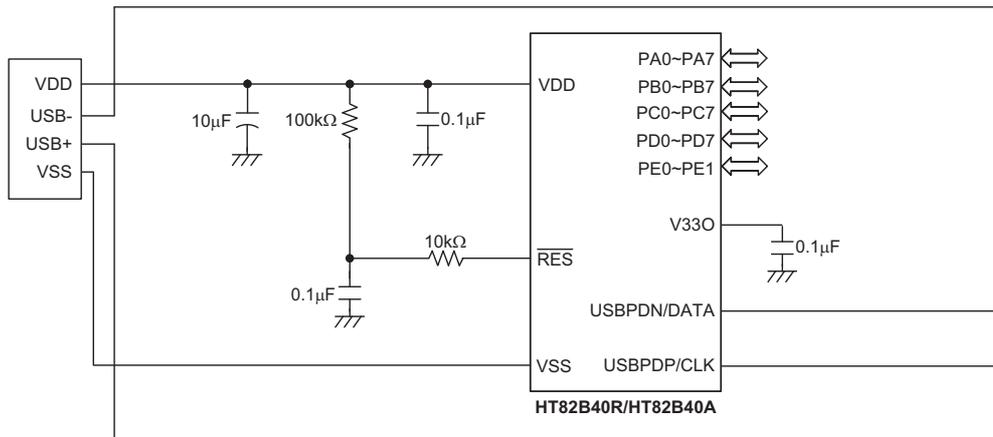
Note: The resistance and capacitance for the reset circuit should be designed in such a way as to ensure that the VDD is stable and remains within a valid operating voltage range before bringing RES high. Components with \* are used for EMC issue.
