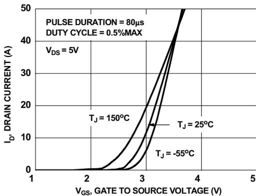
Figure 5. Transfer Characteristics
