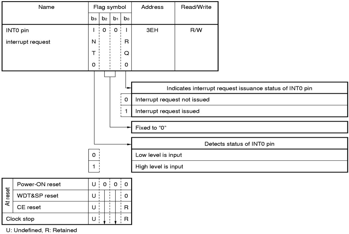
Figure 12-13. Configuration of CE Pin Interrupt Request Register
