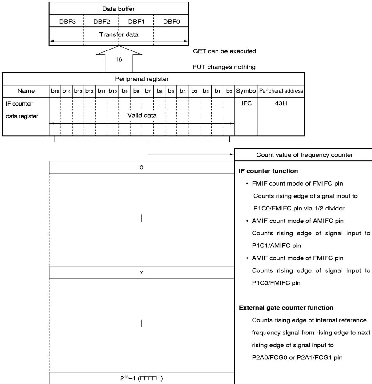
Once the IF counter data register has counted up to FFFFH, it remains at FFFFH until the counter is reset.
