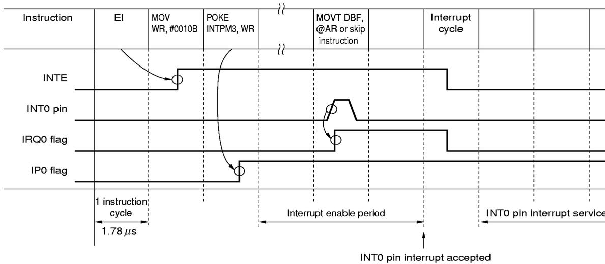
Figure 12-19. Timing Charts When Interrupt Is Accepted (2/3)
