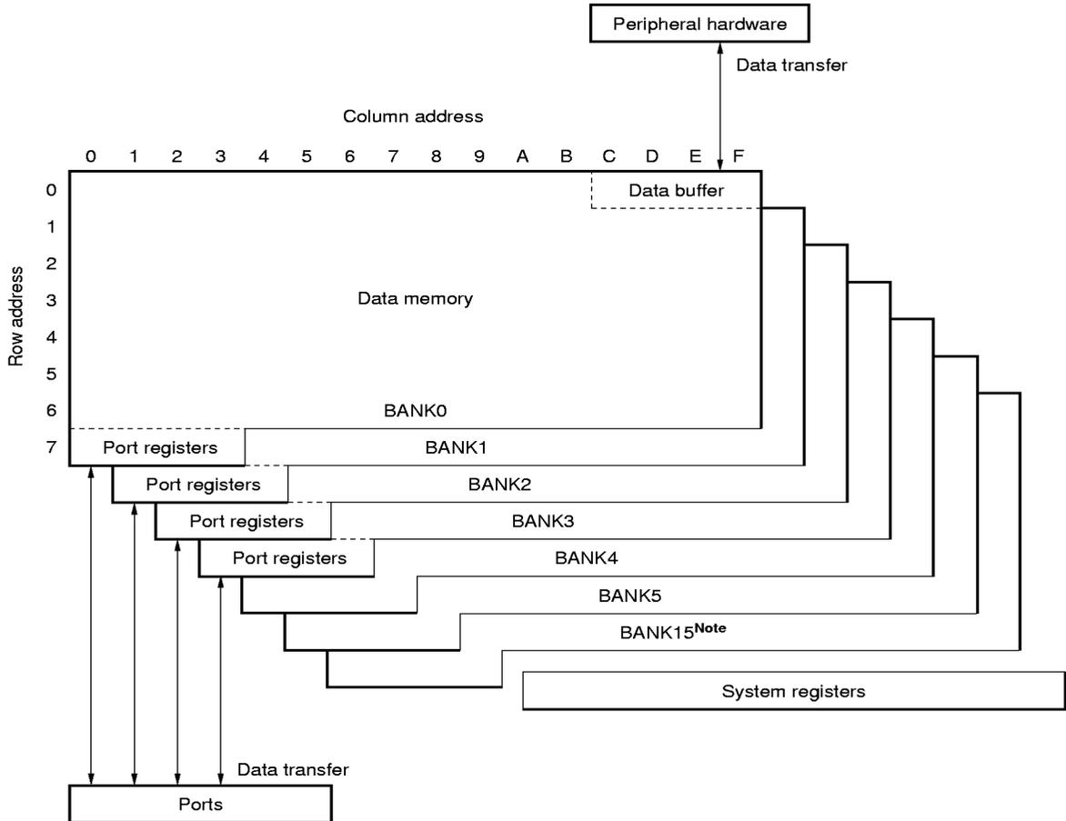
**Note** Port input/output selection registers are allocated to addresses 60H through 6FH of BANK 15.
