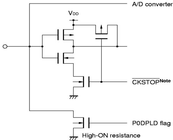
**Note** This is an internal signal that is output when the clock stop instruction is executed, and its circuit is designed not to increase the current consumption due to noise even if it is floated.
