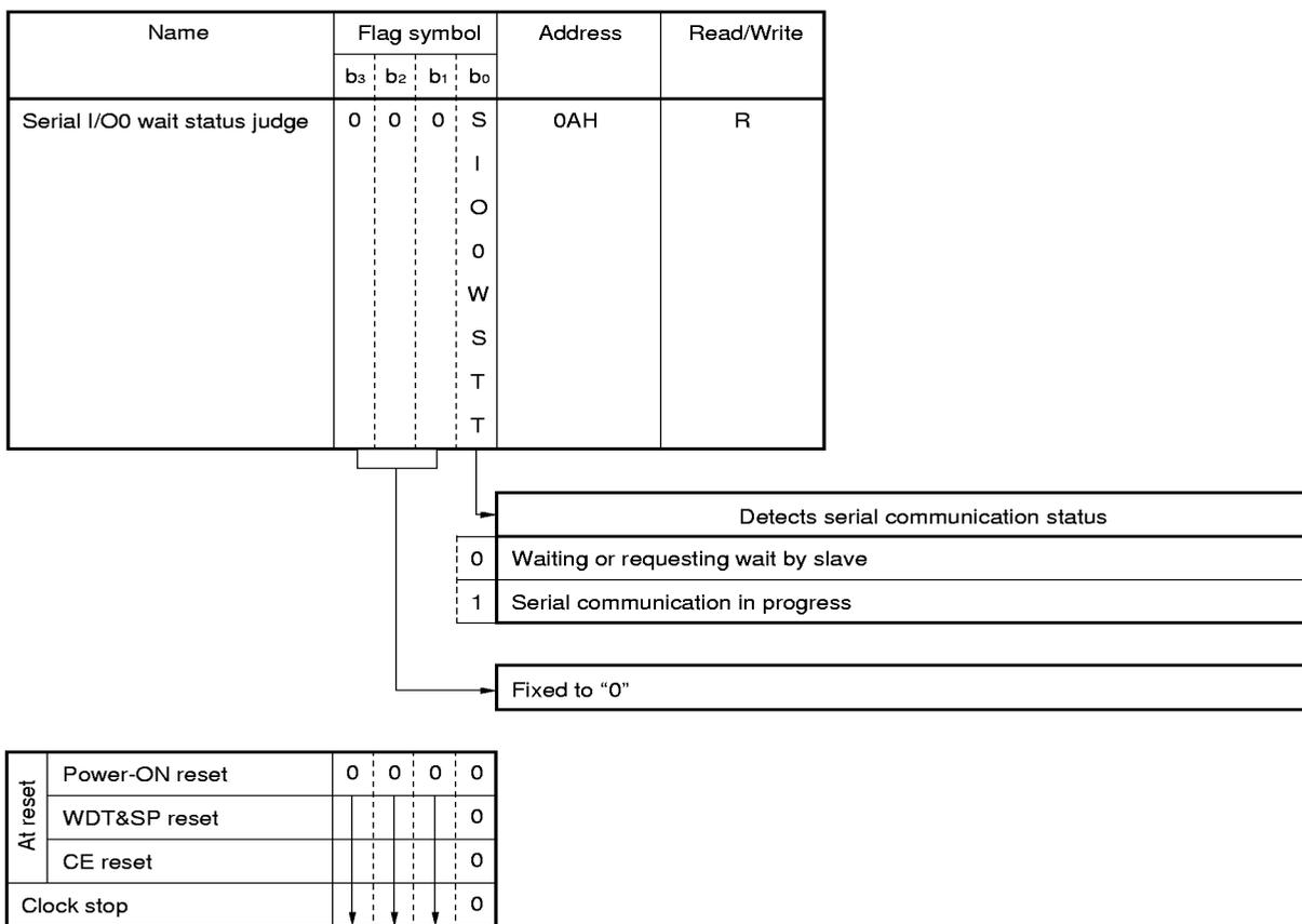
**Caution** If a slave outputs a wait request while the master is operating, "0" is detected on the SIO0WSTT flag. The SIO0NWT flag retains the status of 1.
