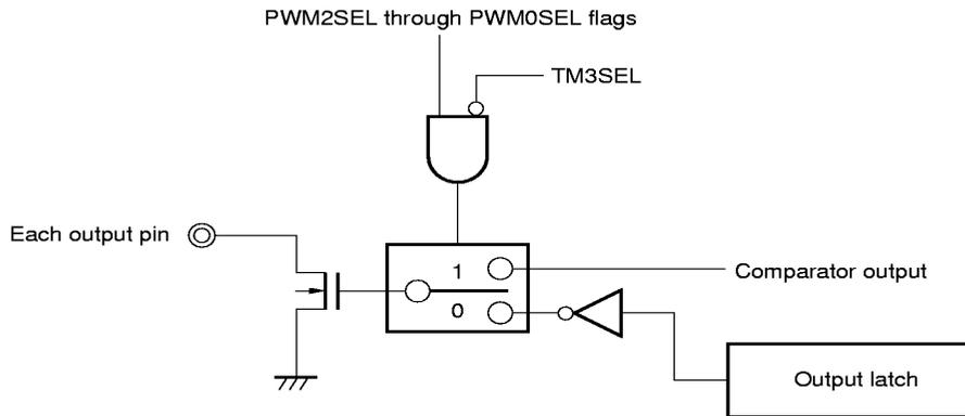
Figure 15-4. Configuration of PWM/General-Purpose Port Pin Function Selection Register
