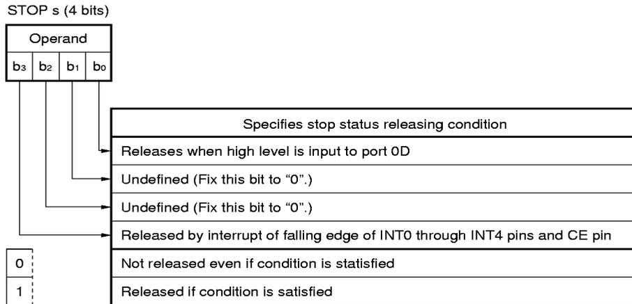
The "STOP s" instruction is executed as a "NOP" instruction when the CE pin rises and when the CE reset counter operates.
