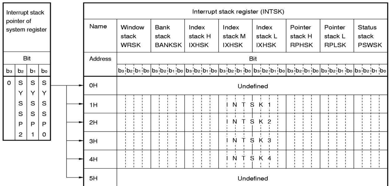
**12.3.2 Interrupt stack pointer of system register**
