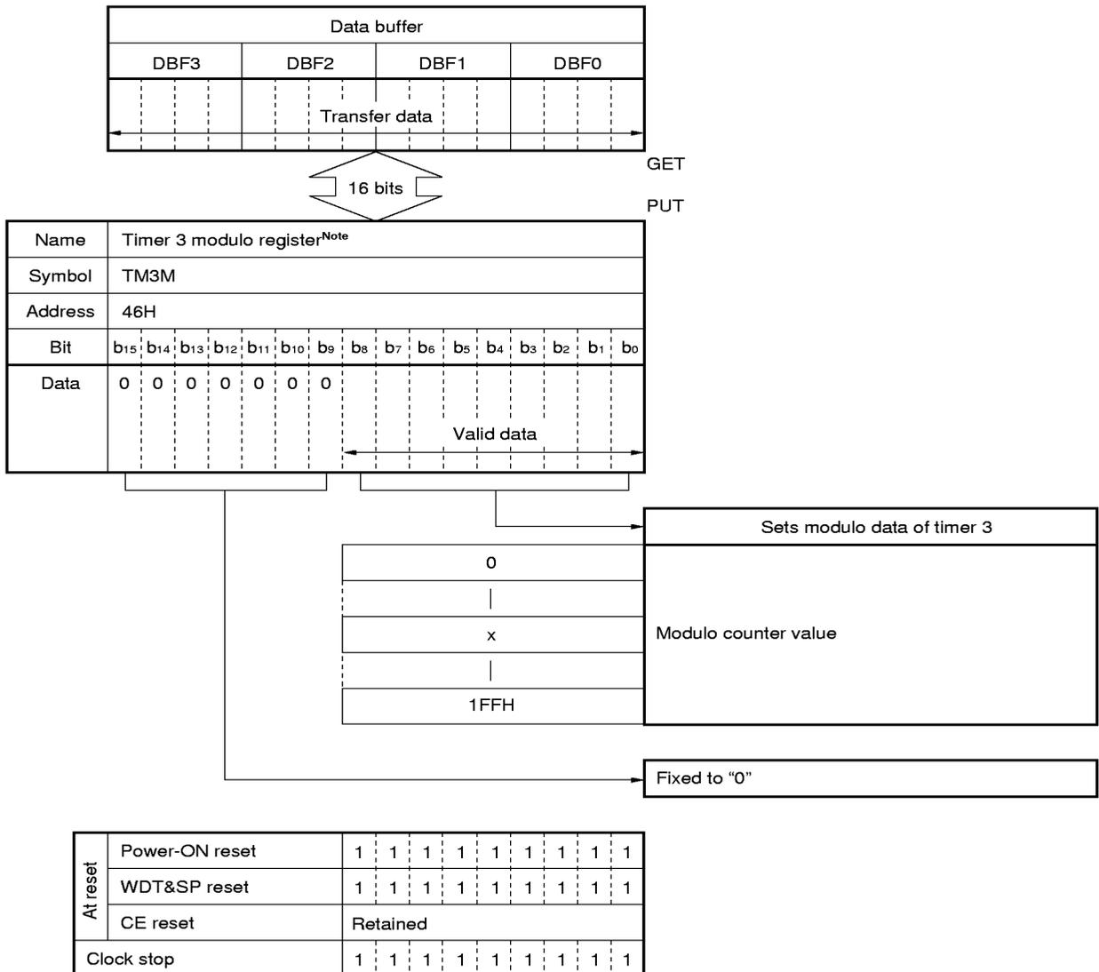
**Note** This register is multiplexed with the PWM data register.
