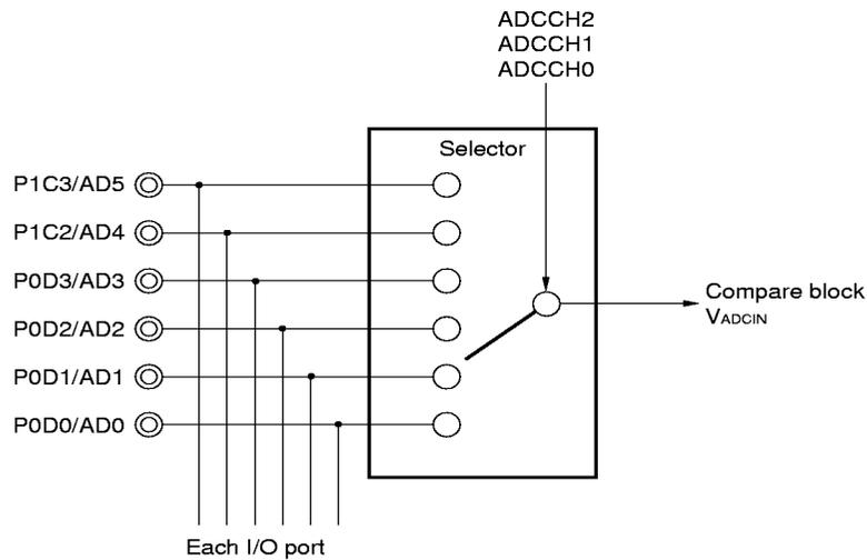
Figure 14-3. Configuration of A/D Converter Channel Selection Register
