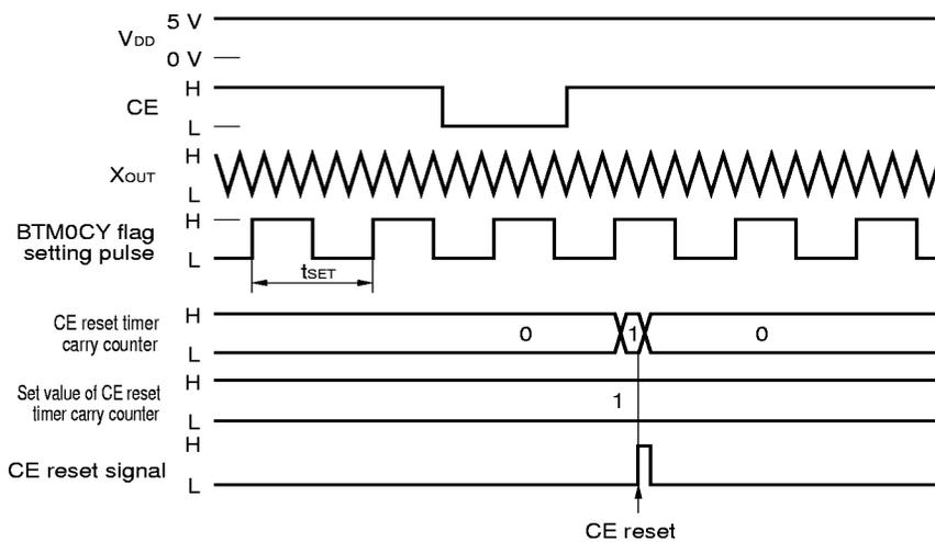
Figure 21-3. CE Reset Operation without Clock Stop Instruction (2/2)
