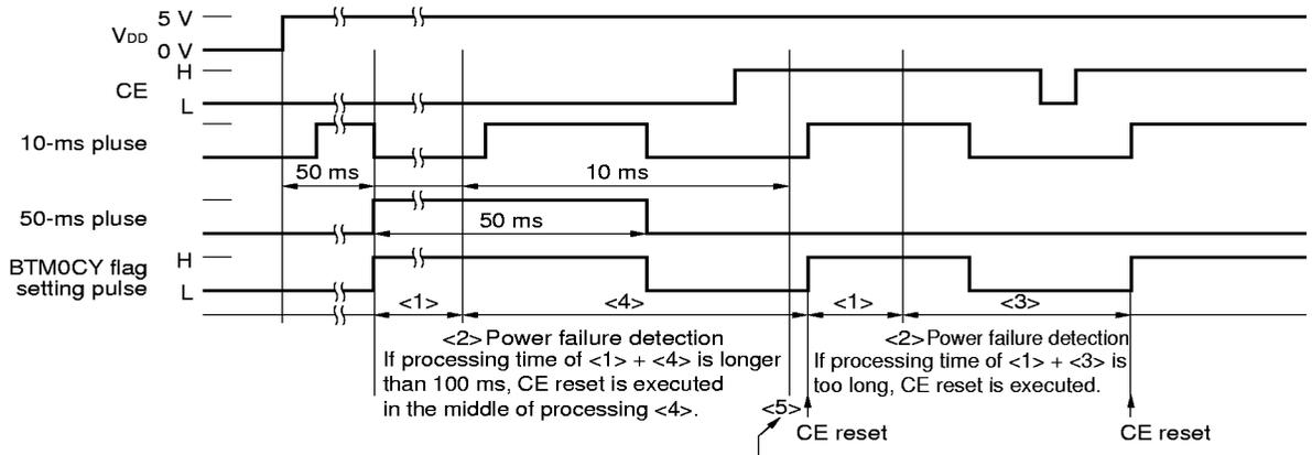
CE reset may be executed immediately depending on when the basic timer 0 carry FF setting time is changed. Therefore, if <5> is executed before <4>, power failure processing <4> may not be executed to the end.
