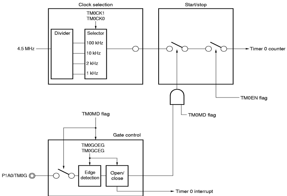
Figure 13-13. Configuration of Timer 0 Counter Clock Selection Register
