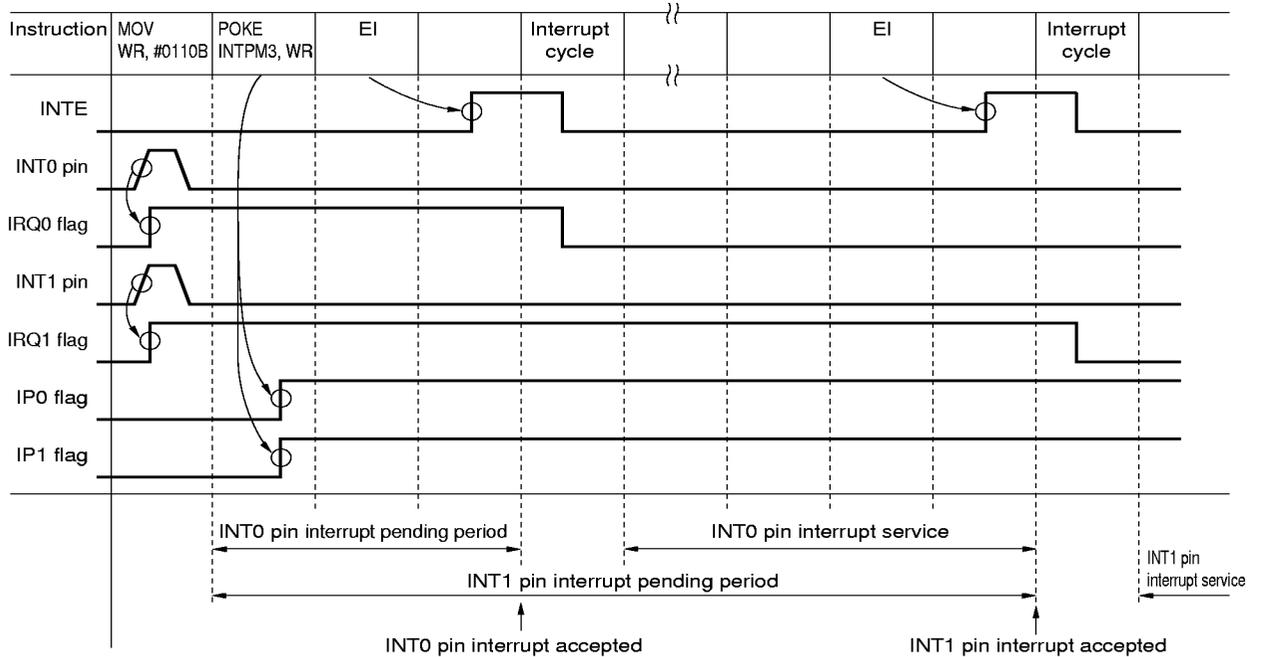
Figure 12-19. Timing Charts When Interrupt Is Accepted (3/3)
