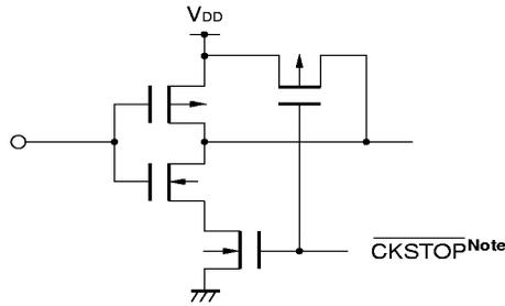
**Note** This is an internal signal output on execution of the clock stop instruction, and its circuit is designed not to increase the current consumption due to noise even if the pin is floated.
