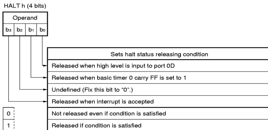
**20.2.4 Releasing halt by input port (P0D)**
