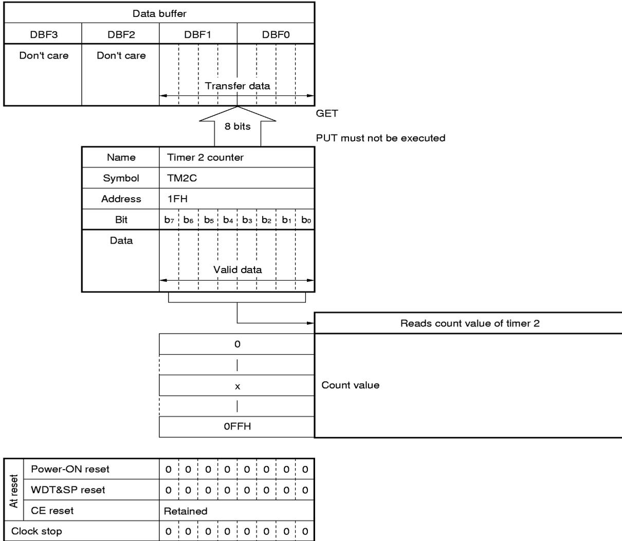
Figure 13-24. Configuration of Timer 2 Modulo Register
