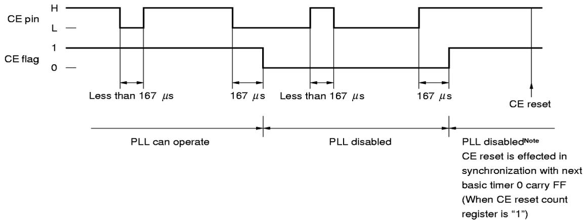
**Note** Unless the PLL mode selection register and PLL reference frequency selection register are rewritten by software, the PLL disabled status is retained.
