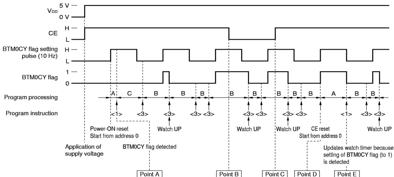
As shown in Figure 13-9, the program is started from address 0000H because the internal 10-Hz pulse rises when supply voltage V<sub>DD</sub> is first applied.
