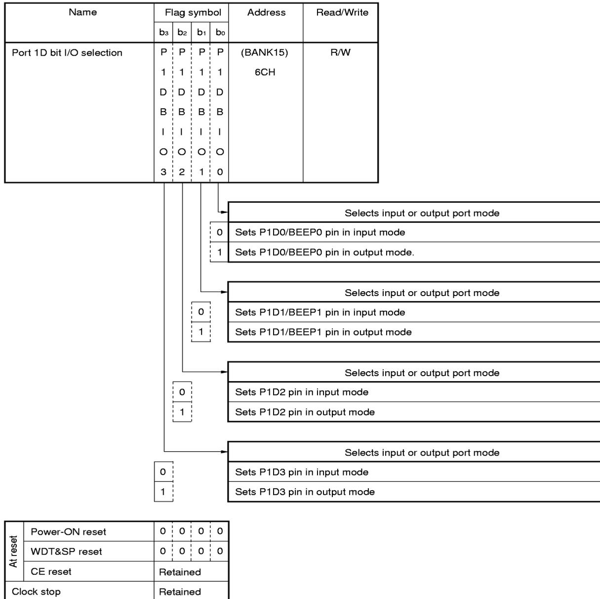
Figure 19-3. Configuration of BEEP/General-Purpose Port Pin Function Selection Register
