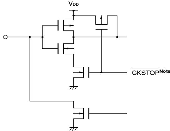
**Note** This is an internal signal that is output when the clock stop instruction is executed, and its circuit is designed not to increase the current consumption due to noise even if it is floated.
