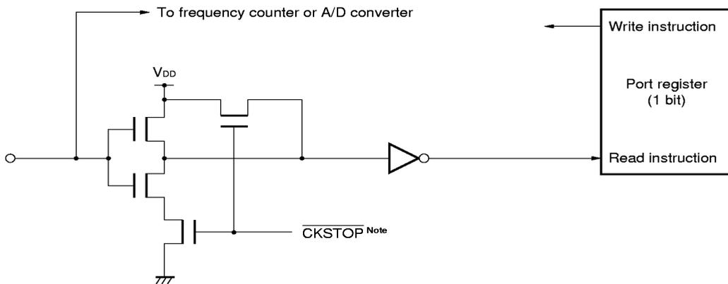
**Note** This is an internal signal output on execution of the clock stop instruction, and its circuit is designed not to increase the current consumption due to noise even if the pin is floated. (Except P1A3, P1A2, P1A0)
