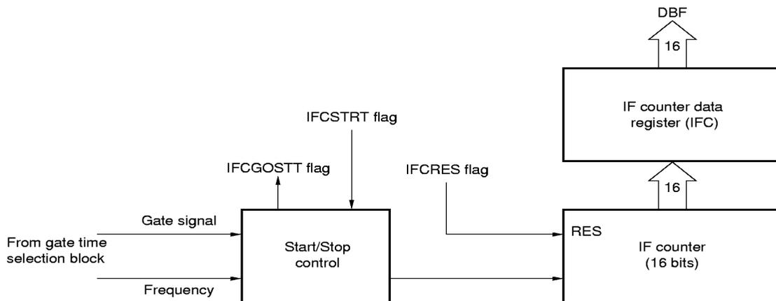
Figure 18-6. Configuration of IF Counter Control Register
