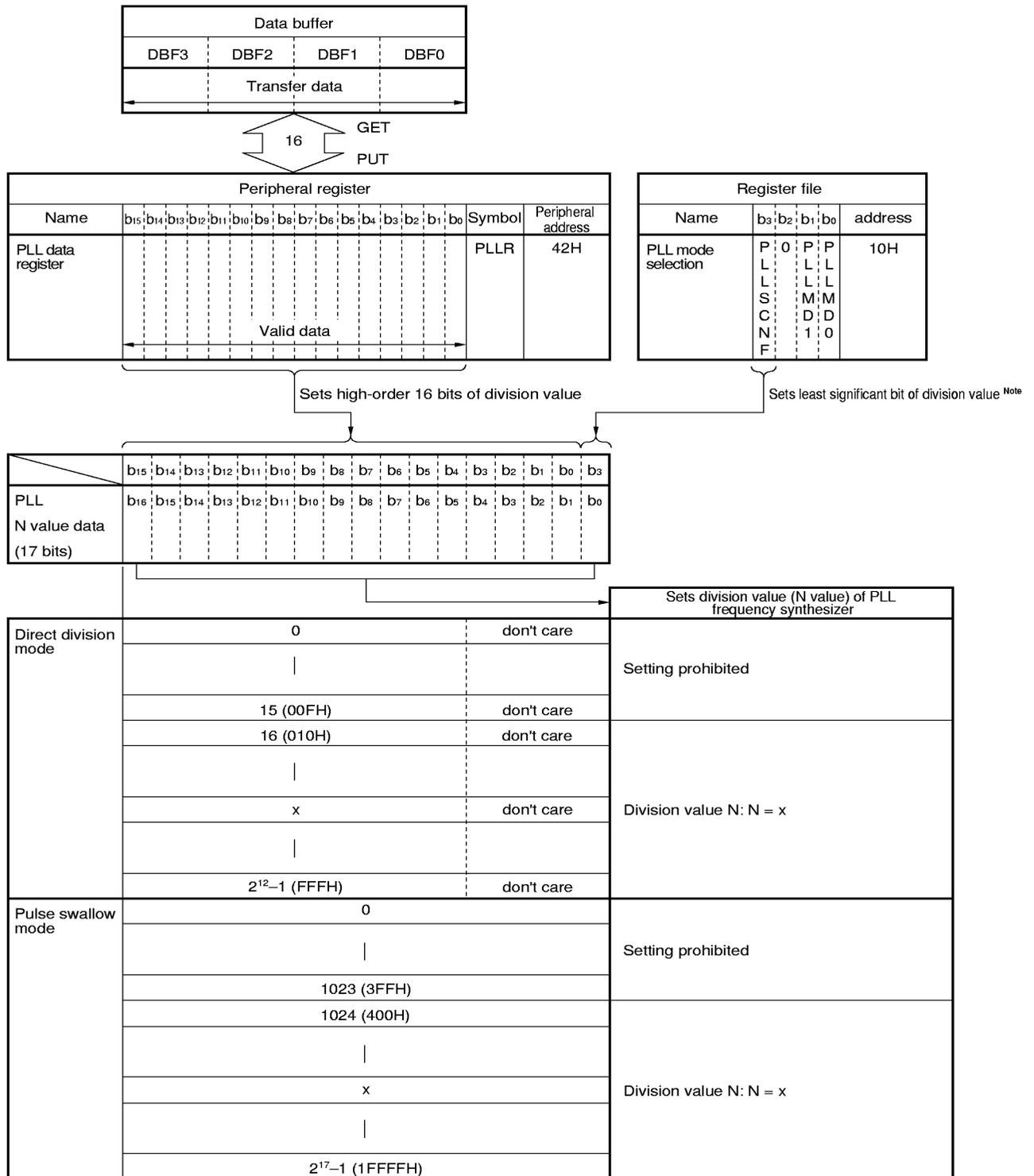
**Note** The value of PLLSCNF flag is transferred when a write (PUT) instruction is executed to the PLL data register (PLL R). Therefore, data must be set to the PLLSCNF flag before executing the write instruction to the PLL data register.
