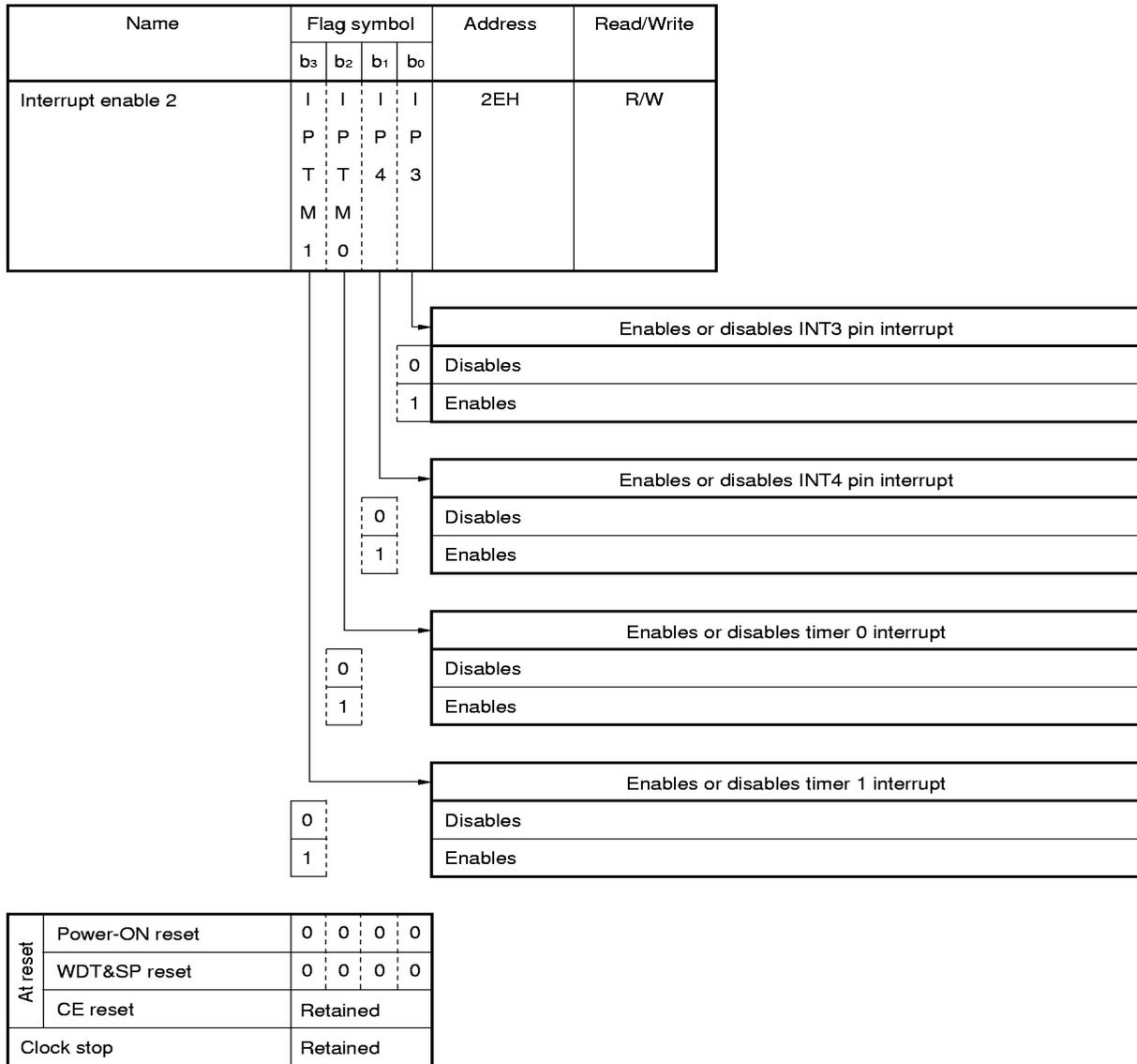
Figure 12-16. Configuration of Interrupt Enable Register 3
