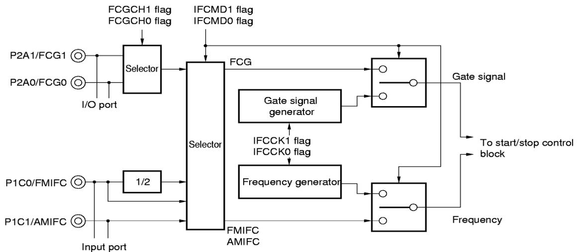
Figure 18-3. Configuration of IF Counter Mode Selection Register
