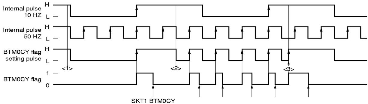
As shown in Figure 13-6, if the BTM0CY flag setting time is changed and the new pulse falls, the BTM0CY flag retains the previous status (<2> in the figure). If the new pulse rises, however, the BTM0CY flag is set to "1" (<3> in the figure).
