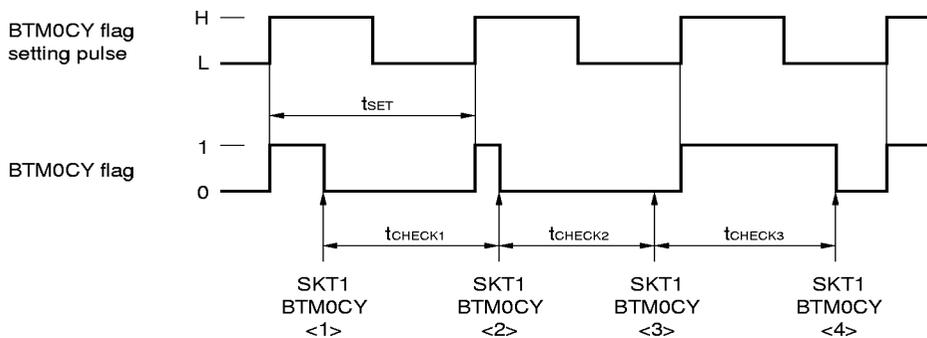
As shown in Figure 13-5, the timer is updated because BTM0CY flag is "1" when it is detected in step <2>.
