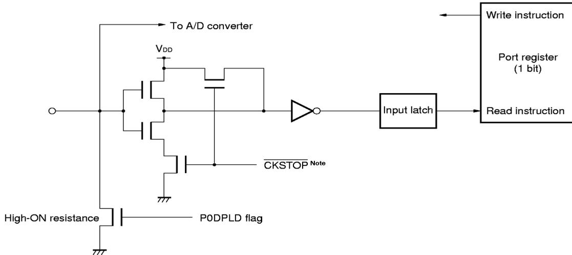
**Note** This is an internal signal output on execution of the clock stop instruction, and its circuit is designed not to increase the current consumption due to noise even if the pin is floated.
