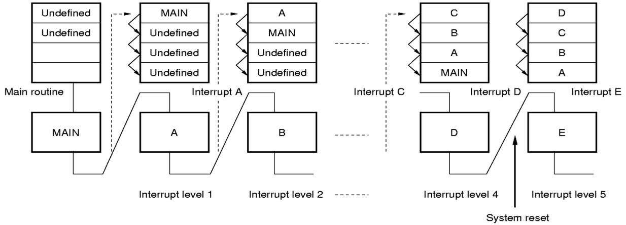
**Caution** The system is reset when an interrupt of level 5 is accepted. However, the ISPRES flag, which resets the non-maskable interrupt if the interrupt stack overflows or underflows, must be set to "1". This flag is "1" after system reset, and can then be written only once.
