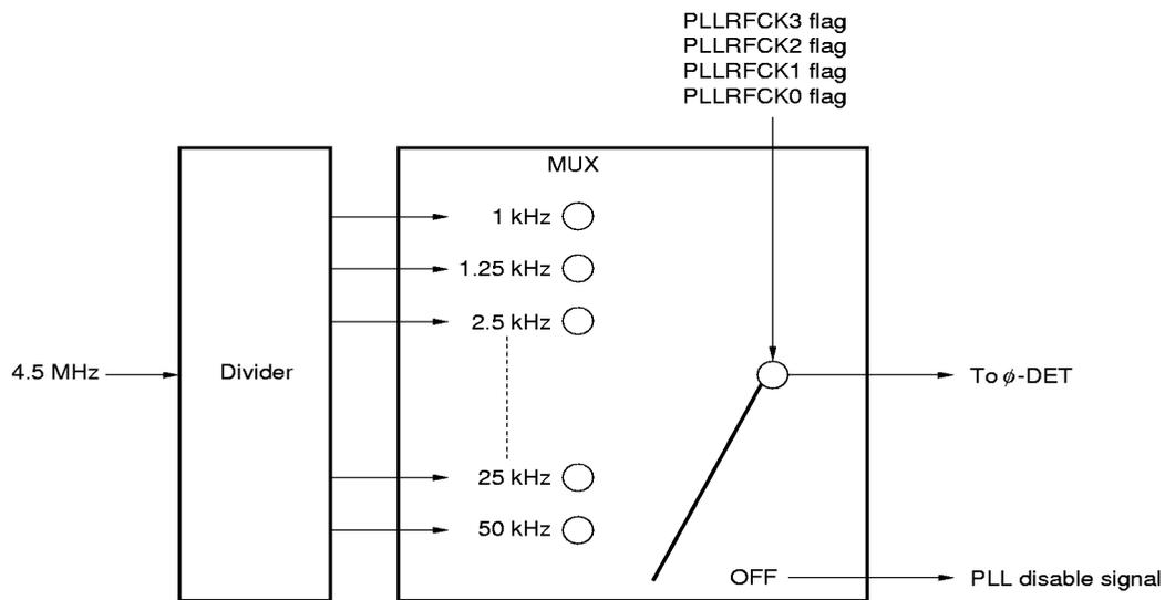
Figure 17-6. Configuration of PLL Reference Frequency Selection Register
