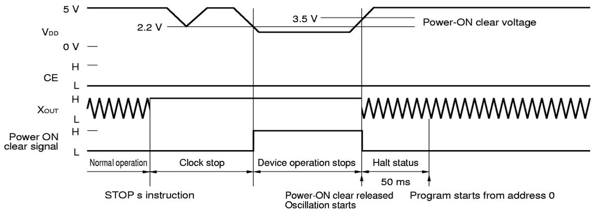
(c) If supply voltage  $V_{DD}$  rises from 0 V
