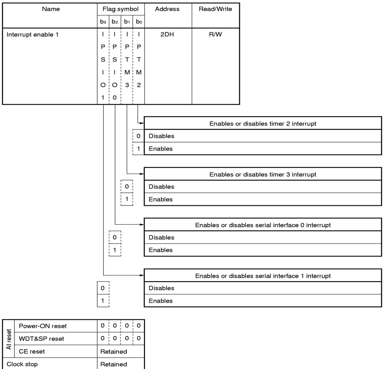
Figure 12-15. Configuration of Interrupt Enable Register 2
