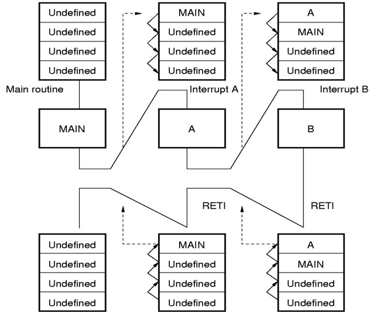
Figure 12-18. Operation of Interrupt Stack (2/2)
