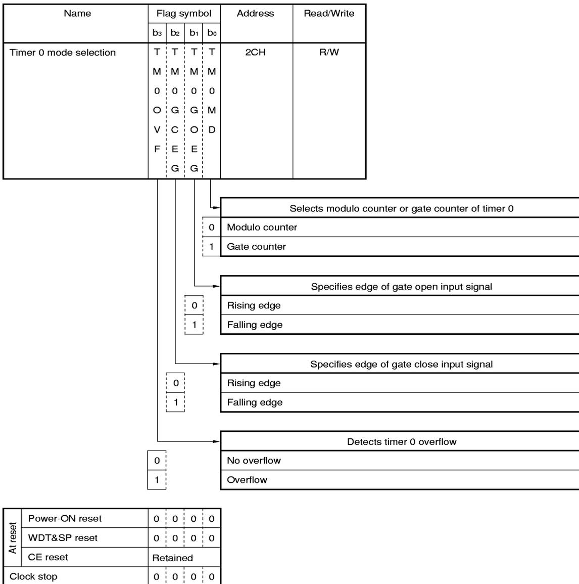
Figure 13-15. Configuration of Timer 0 Counter
