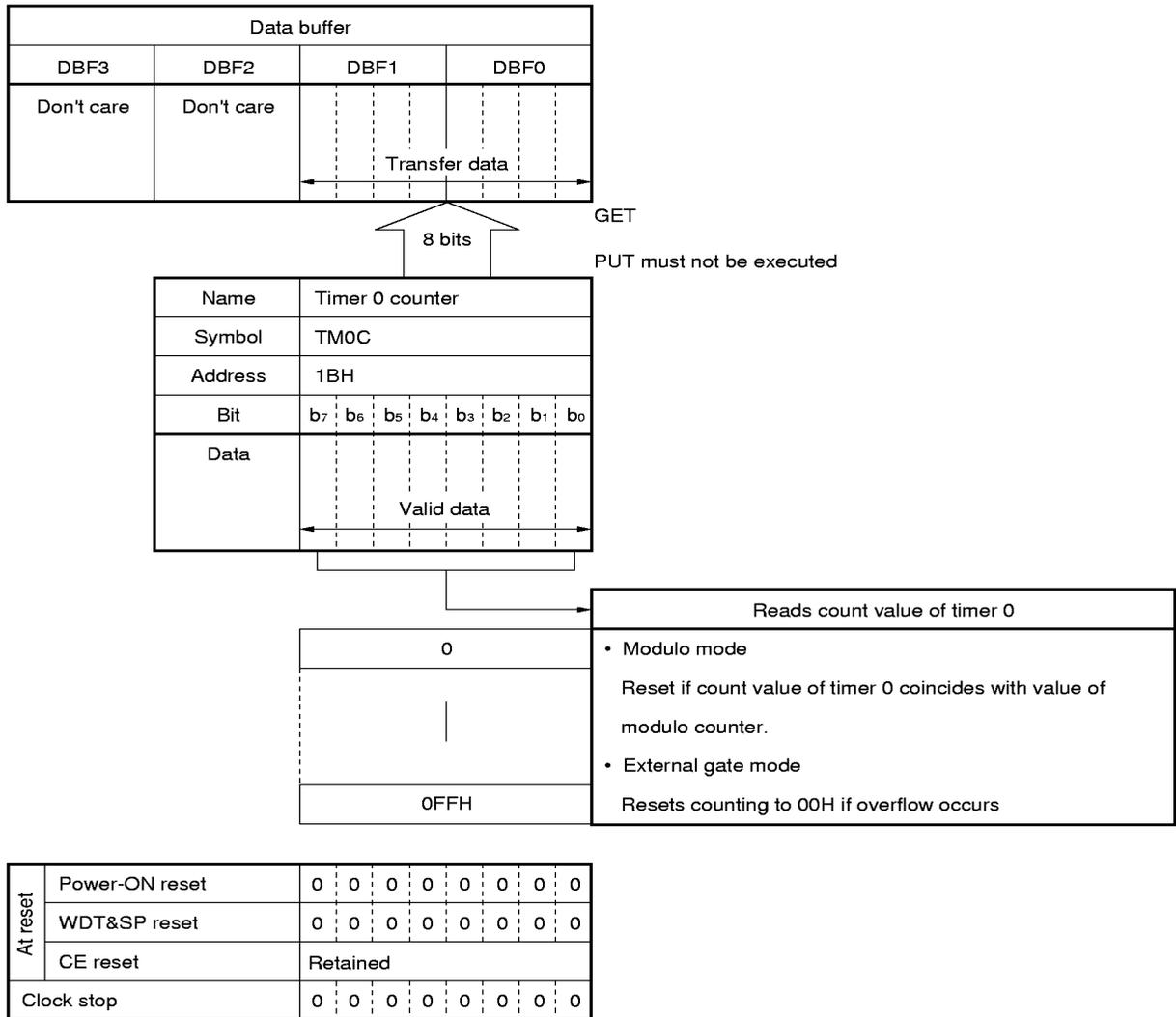
Figure 13-16. Configuration of Timer 0 Modulo Register
