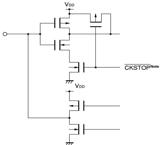
**Note** This is an internal signal that is output when the clock stop instruction is executed, and its circuit is designed not to increase the current consumption due to noise even if it is floated.
