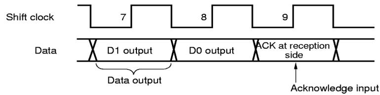
(7) Shift clock generation timing in I<sup>2</sup>C bus mode
