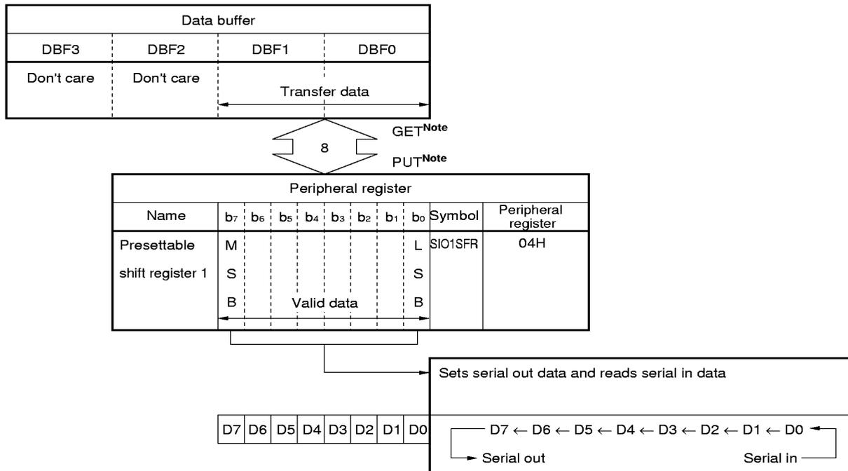
**Note** Data may be destroyed if the PUT or GET instruction is executed during serial communication. For details, refer to **16.3.7 Cautions on setting and reading data.**
