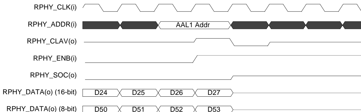
Figure 90 UI_SRC_INTF End-of-Transfer Timing (Utopia 2 PHY Mode)
