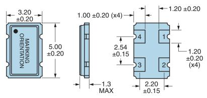
Note: Pin 1 Chamfer not shown.
