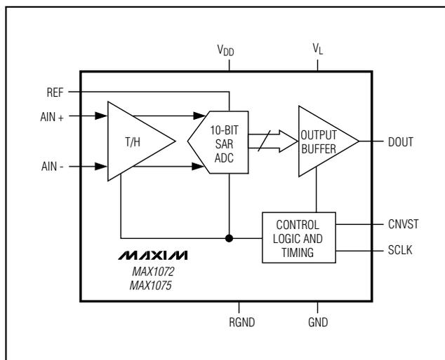
Figure 3. Functional Diagram
