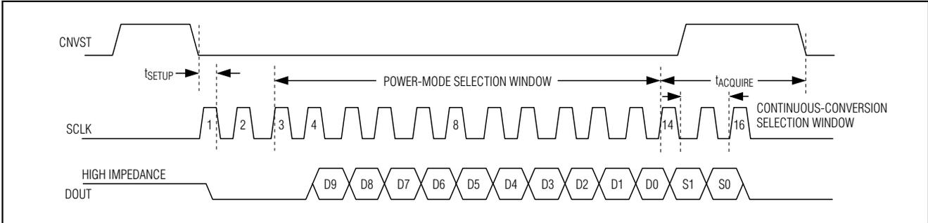
Figure 5. Interface-Timing Sequence
