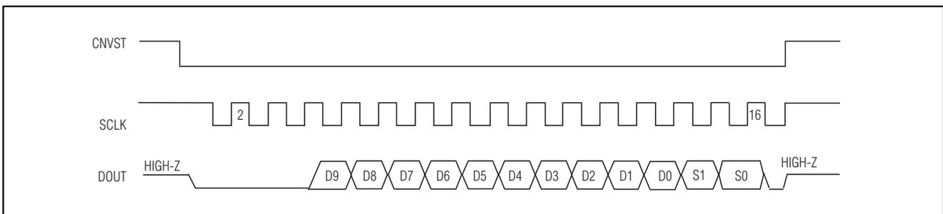
Figure 14. QSPI Serial-Interface Timing—Single Conversion (CPOL = 1, CPHA = 1)
