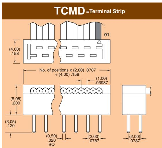
\*Note: Standard TCMD callout will not mate with SMM, MMS. Must use gold plated callouts. (See drawing on web.) When mated with a socket, Wire 1 mates with Pin 2; Wire 2 mates with Pin 1, etc.
