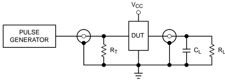
$C_L = 50$  pF at  $V_{CC} = 3.3 \pm 0.3$  V or equivalent (includes jig and probe capacitance)
