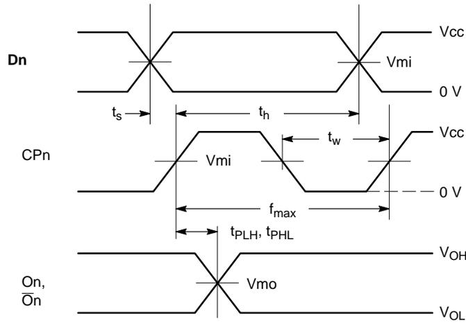
**WAVEFORM 1 – PROPAGATION DELAYS, SETUP AND HOLD TIMES**
