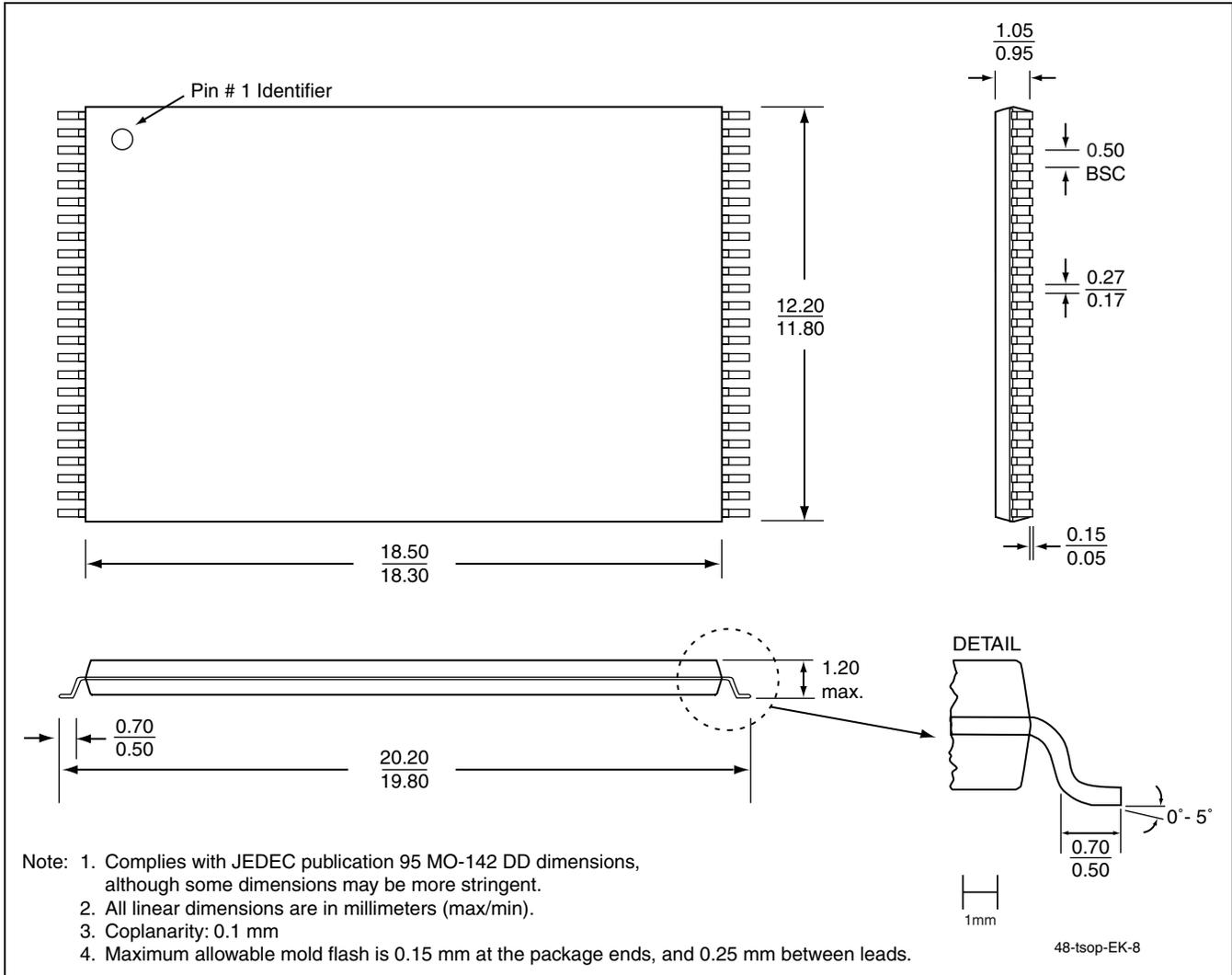
**48-LEAD THIN SMALL OUTLINE PACKAGE (TSOP) 12MM X 20MM**
