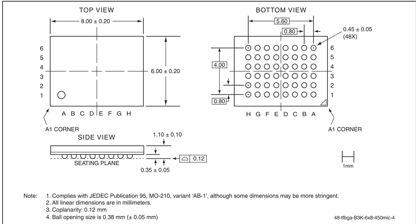
**48-BALL THIN-PROFILE, FINE-PITCH BALL GRID ARRAY (TFBGA) 6MM X 8MM**
