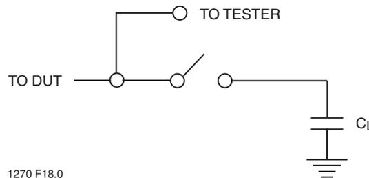
FIGURE 19: A Test Load Example
