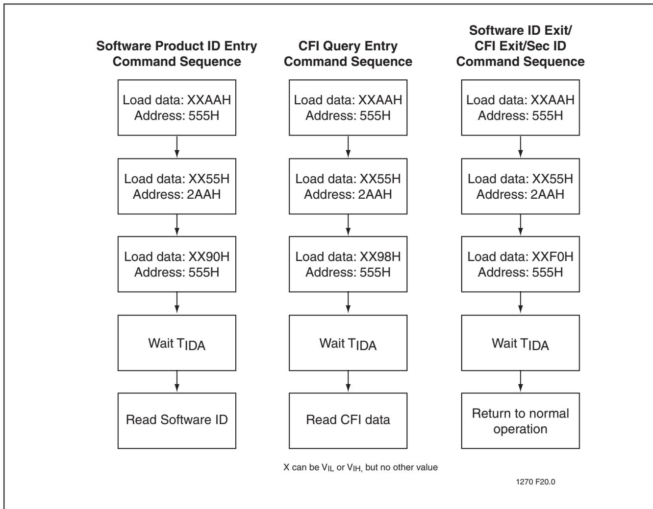
FIGURE 22: Software Product ID/CFI/Sec ID Entry Command Flowcharts
