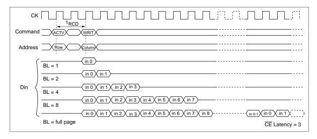
**2. Single write:** A single write operation is enabled by setting OPCODE (A9, A8) to (1, 0). In a single write operation, data is only written to the column address and the bank select address (BA) specified by the write command set cycle without regard to the burst length setting. (The latency of data input is 0 clock).
