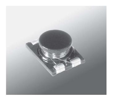
The DW3316 features a unique dual winding configuration that provides two balanced coupled inductors in a single package. This increases circuit efficiency, reduces component count and conserves valuable board space. Interwinding isolation for this part is 500 Vrms.
