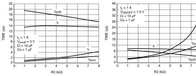
Figure 8. Switching Variation R2 @  $V_{in}$  = 4.5 V, R1 = 20 k $\Omega$
