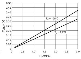
Figure 2.  $V_{drop}$  vs.  $I_L @ V_{in} = 2.5 \text{ V}$
