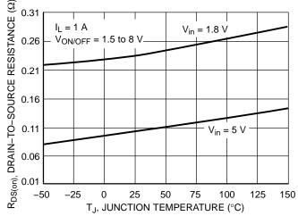
Figure 4. On-Resistance vs. Input Voltage
