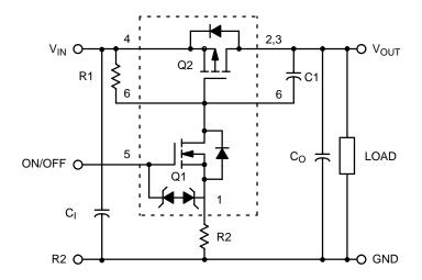
Figure 1. Load Switch Application
