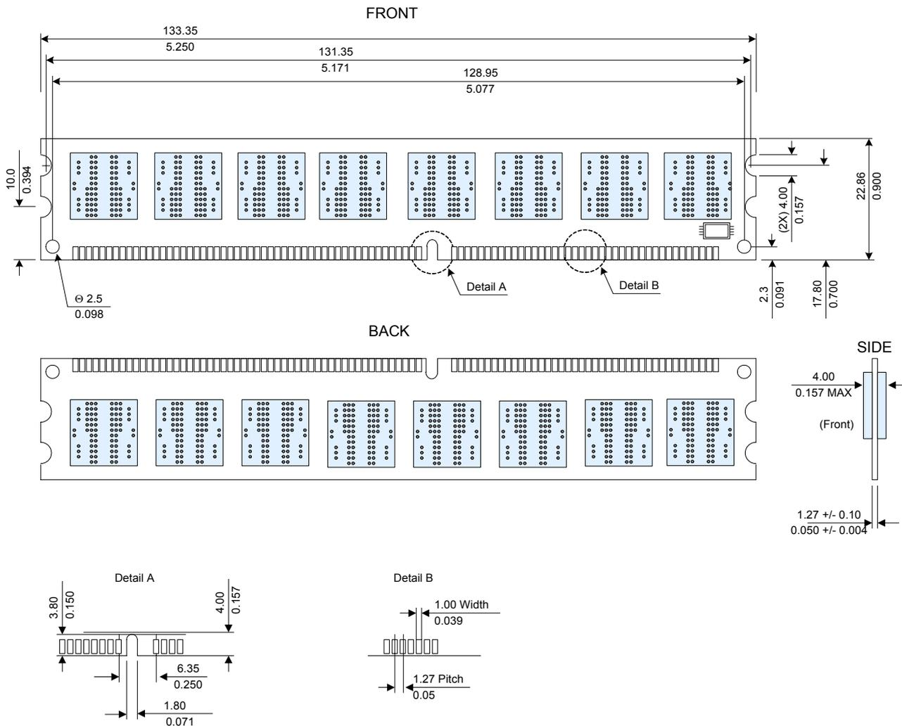
Note: All dimensions are typical with tolerances of +/- 0.15 (0.006) unless otherwise stated.
