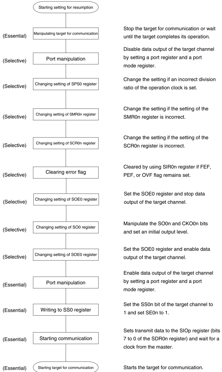
Figure 12-48. Procedure for Resuming Slave Transmission
