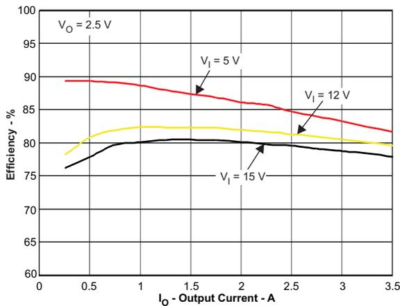
Figure 14. TPS54332 Efficiency
