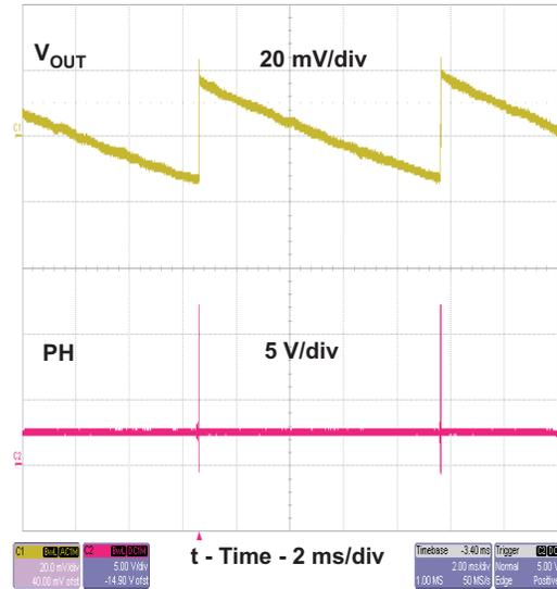
Figure 23. TPS54332 Output Ripple During Eco-mode™ Operation
