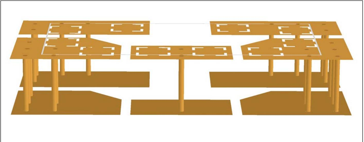
**Figure 5** – Recommended mounting on a 2 layer board
