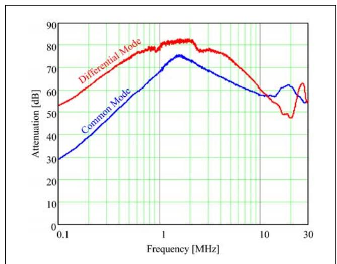
Figure 3 – QPI-11 network analyzer attenuation curves
