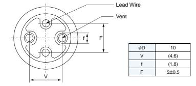
Products of vent on rubber type, please make clearance about 1mm minimum between rubber and board. If it is difficult to make clearance 1mm minimum between rubber and board, please arrange gas escaping hole on the board (same position and 40% minimum diameter from the vent).
