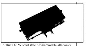
Trilithic's NEW solid state programmable attenuator model PA-1527-1 operates from 400 to 2000 MHz. The attenuation range is 0–127 dB in 1 dB steps. The switching speed is 2 microseconds. The operating supply voltage is 5 volts, and is controlled with TTL. This unit was designed and manufactured for customers in the PCS and Wireless Telephony markets. Many customers use this product in simulation lab environments or GPS testing applications.
