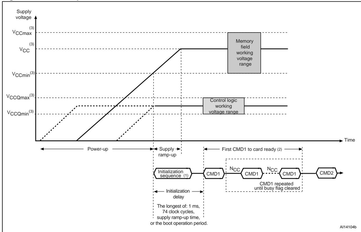
1. The initialization sequence is a contiguous stream of logic 1's. Its length is either 1 ms, 74 clocks or the supply ramp up time, whichever is the longest. The device shall complete its initialization within 1 second from the first CMD1 with a valid V range.
