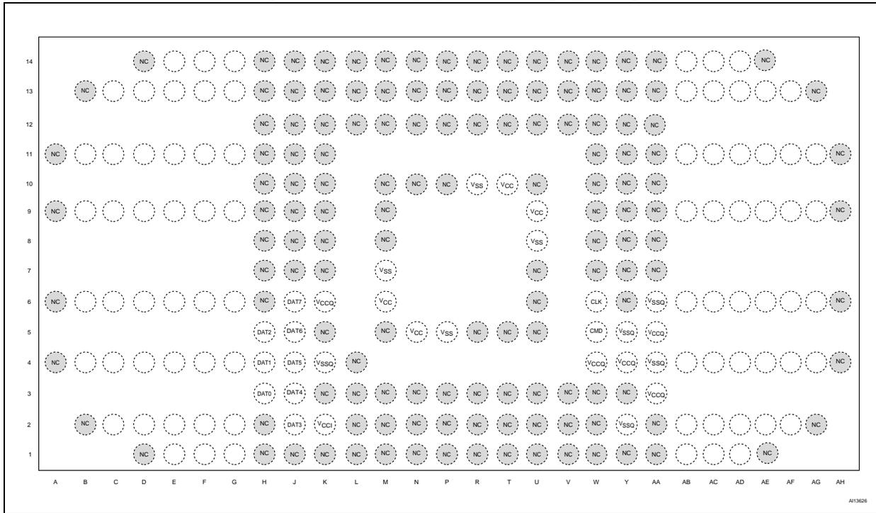
1. The ball corresponding to  $V_{CC1}$  must be decoupled with an external capacitance.
