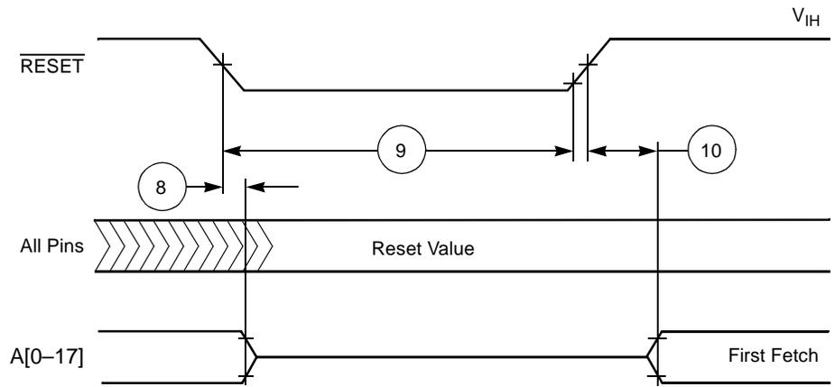
Figure 2-3. Reset Timing
