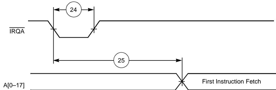
Figure 2-7. Recovery from Stop State Using  $\overline{\text{IRQA}}$
