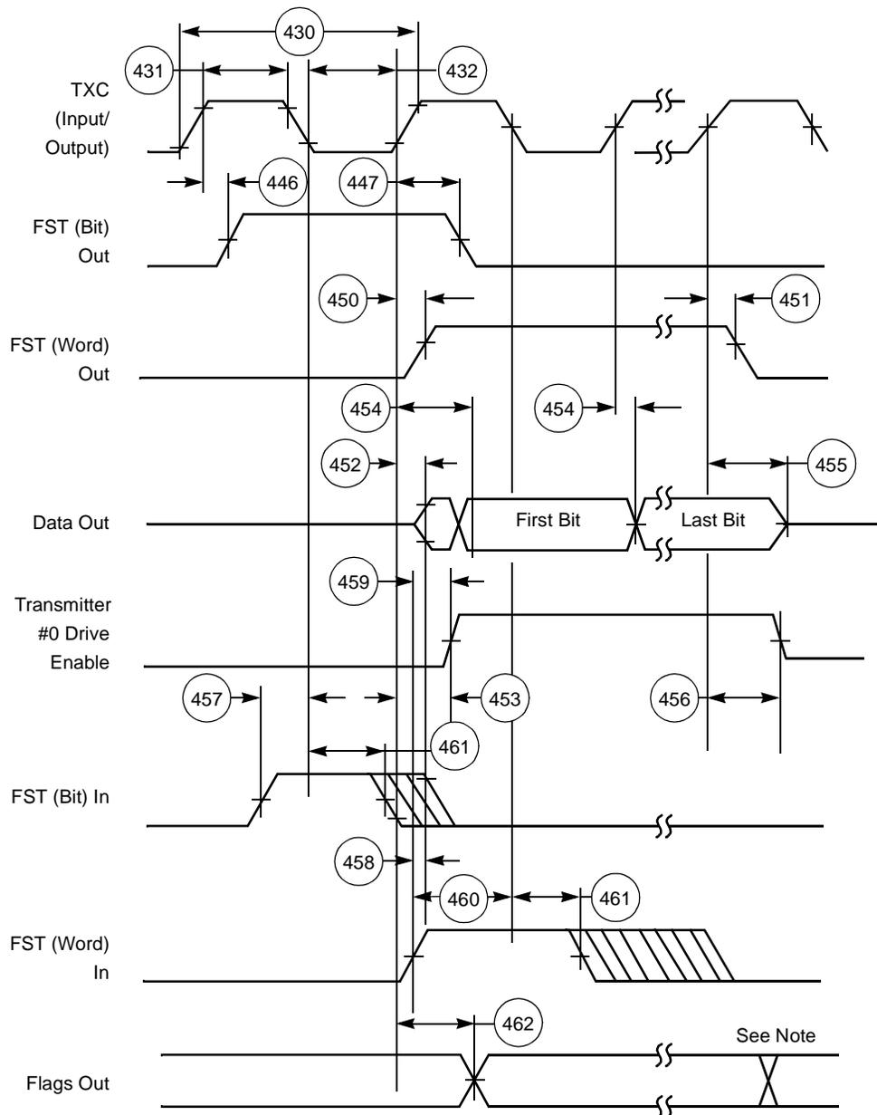
**Note:** In Network mode, output flag transitions can occur at the start of each time slot within the frame. In Normal mode, the output flag state is asserted for the entire frame period.
