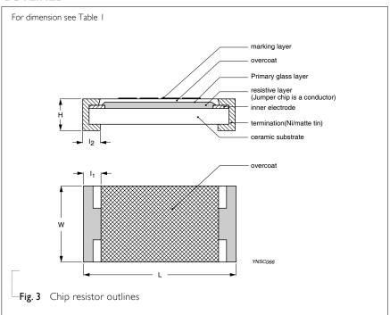
Chip Resistor Surface Mount RC SERIES 1206 (RoHS Compliant)
