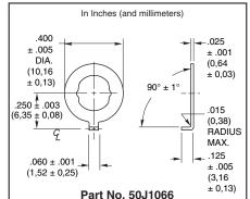
Cut round hole for the bushing and for the non-turn tab. Washer fits the double D bushing flats. Washer is sold only when accompanied by an order for a like number of switches. Washer is 302 stainless steel.
